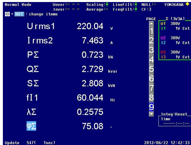
Figure 4.2: No Load Test Data
