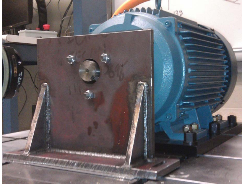
Figure 4.3: Rotor Blocking Fixture
