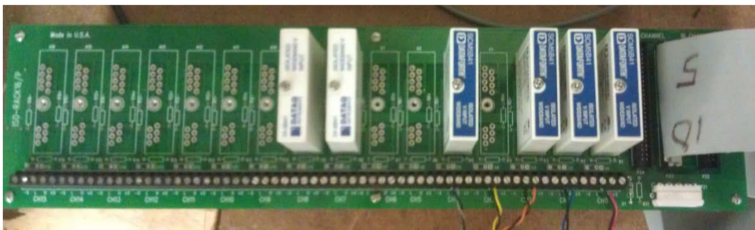
Figure 3.11: Signal Isolation Module Chassis
