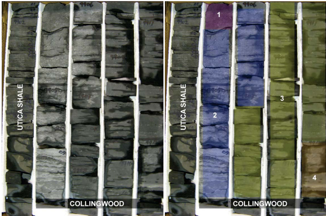
Figure 4.1: Well core section (left) with four distinct facies highlighted (right). Hunt Energy Corporation, Winterfield Deep Unit A1 (API: 21-035-33680-0100), Clare County, MI.
