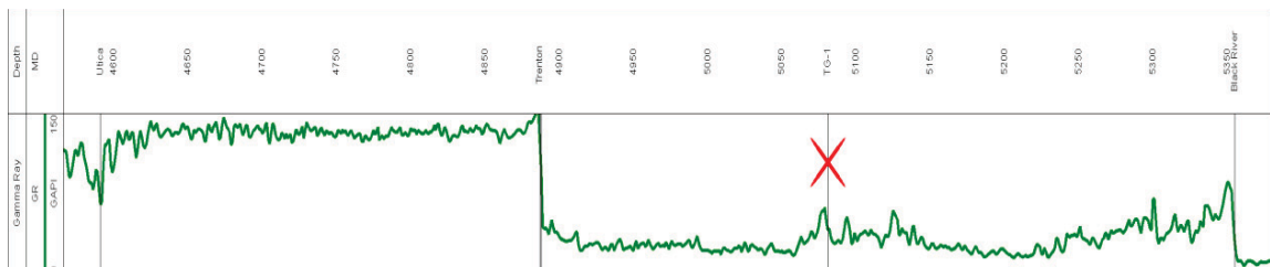
Figure 8.1: Typical Trenton Gamma-Ray Signature showing TG-1 (as indicated by red X), from Miller Bros. & Atlantic Richfield, Arcon & Patton 1-34 (API: 21-147-38965-0000), St. Clair County, MI.
