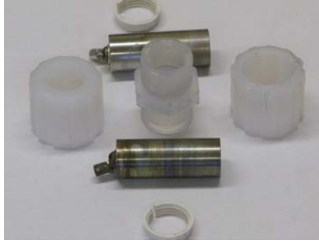
Figure 3.1. The components of a Swagelok-type PFA cell (photograph by author).
