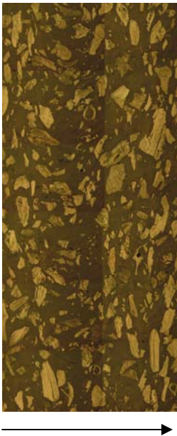
Figure 4.5-2: Through -Plane Thermal Conductivity Sample Containing 40 wt% Calcined Needle Coke F108A in Vectra A950RX at 100X Magnification
