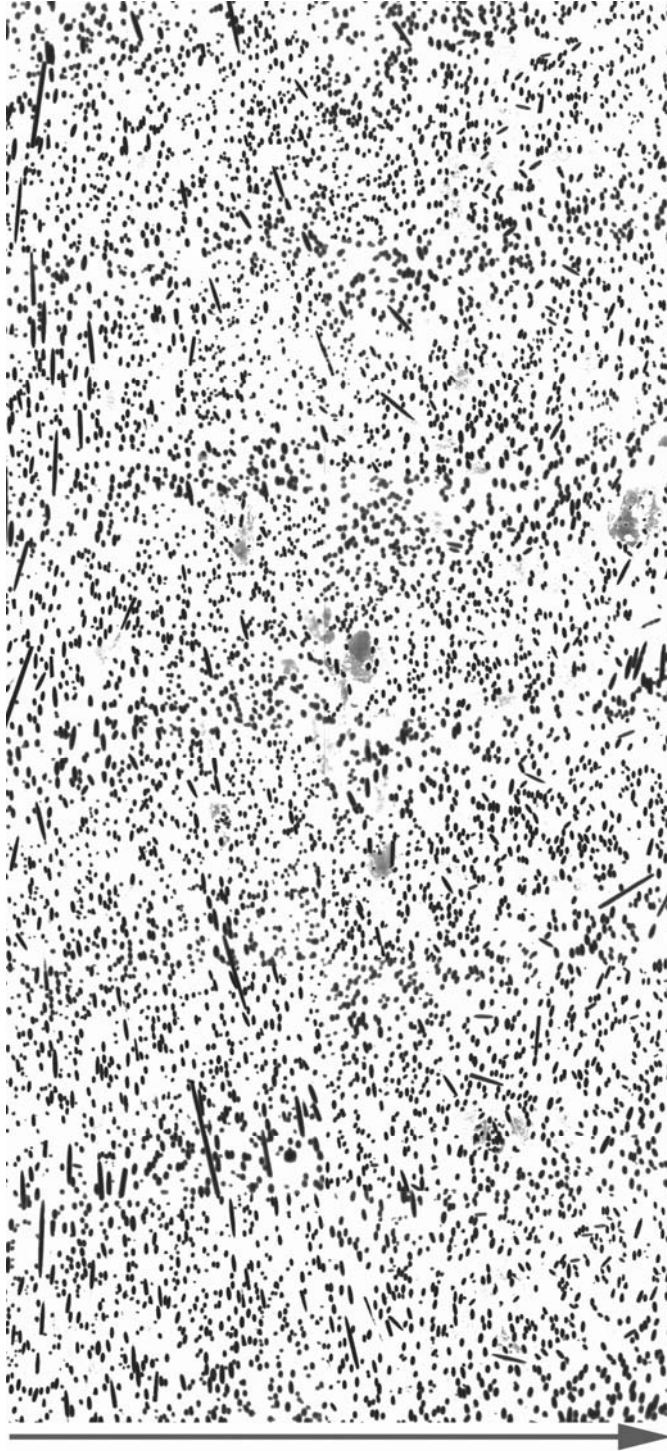
Figure 9.9-14: Optical Micrograph by reflected light of a through-plane thermal conductivity sample containing 20 wt% Fortafil 243 carbon fiber in Vectra A950RX LCP at 100x magnification.
