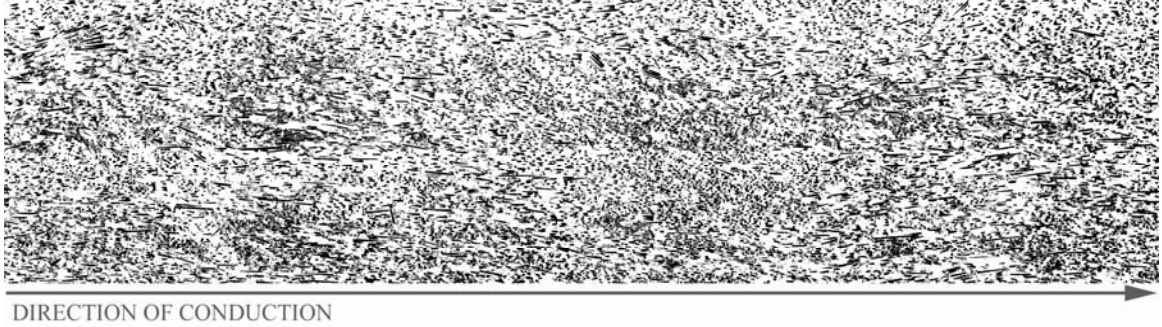
Figure 9.10-16: Optical Micrograph by reflected light of an in-plane electrical resistivity sample containing 60 wt% Fortafil 243 carbon fiber in Vectra A950RX LCP at 100x magnification.
