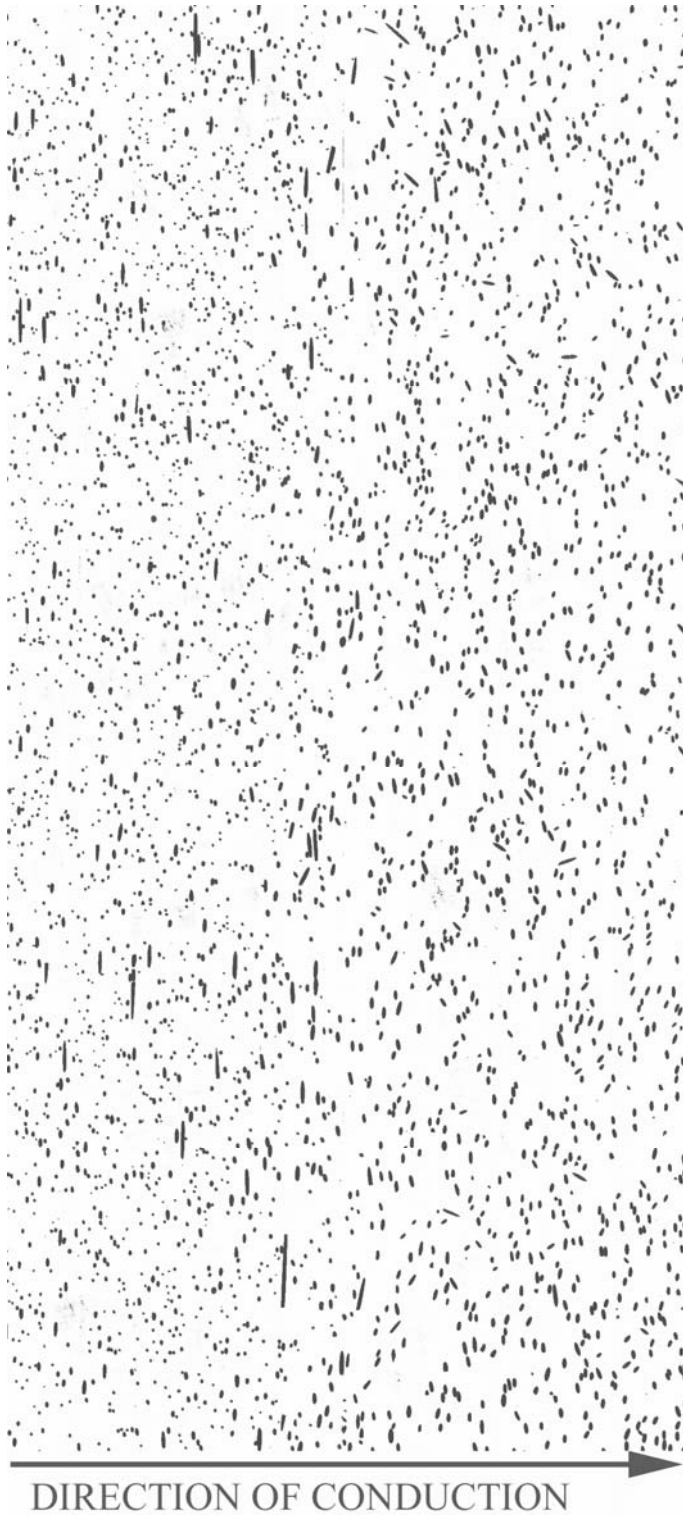
Figure 9.9-13: Optical Micrograph by reflected light of a through-plane thermal conductivity sample containing 10 wt% Fortafil 243 carbon fiber in Vectra A950RX LCP at 100x magnification.
