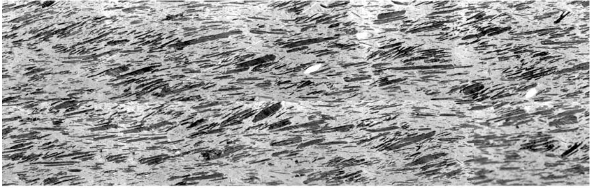
Figure 9.10-7: Optical Micrograph by reflected light of an in-plane electrical resistivity sample containing 40 wt% Asbury 3160 natural flake graphite in Vectra A950RX LCP at 200x magnification.
