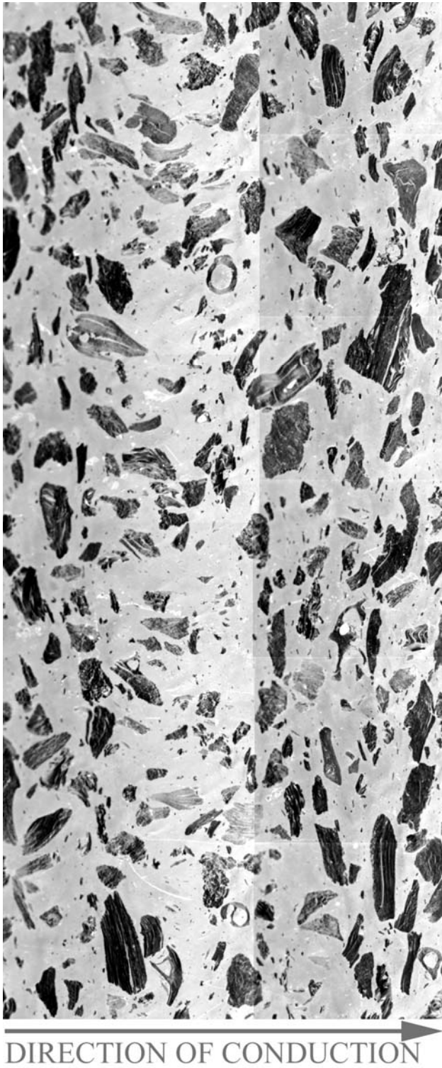
Figure 9.9-10: Optical Micrograph by reflected light of a through-plane thermal conductivity sample containing 40 wt% Asbury F108A CNC in Vectra A950RX LCP at 100x magnification.
