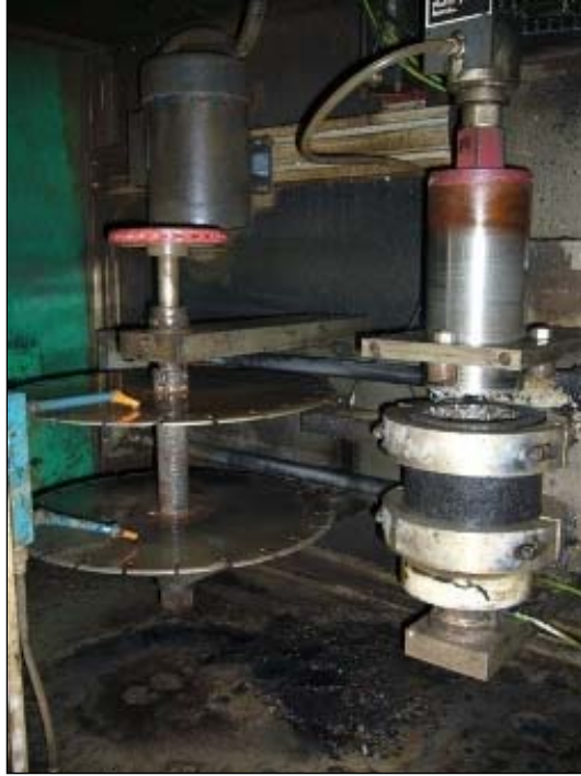
Figure 19 Cutting and Coring Process
