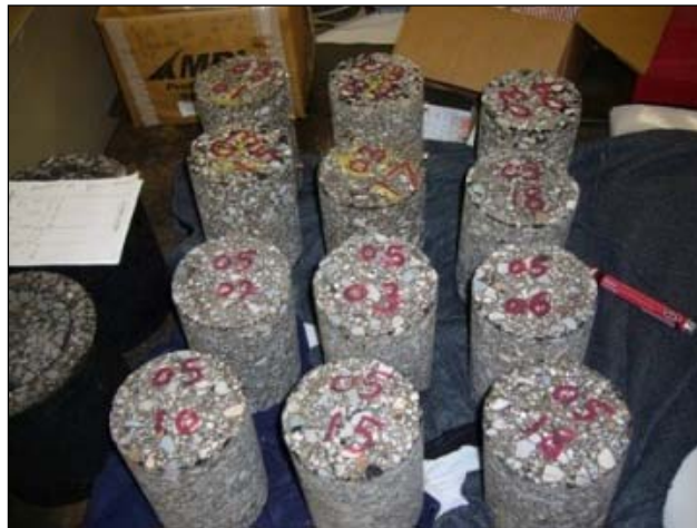
Figure 20 Asphalt Mixture after Cutting and Coring process
