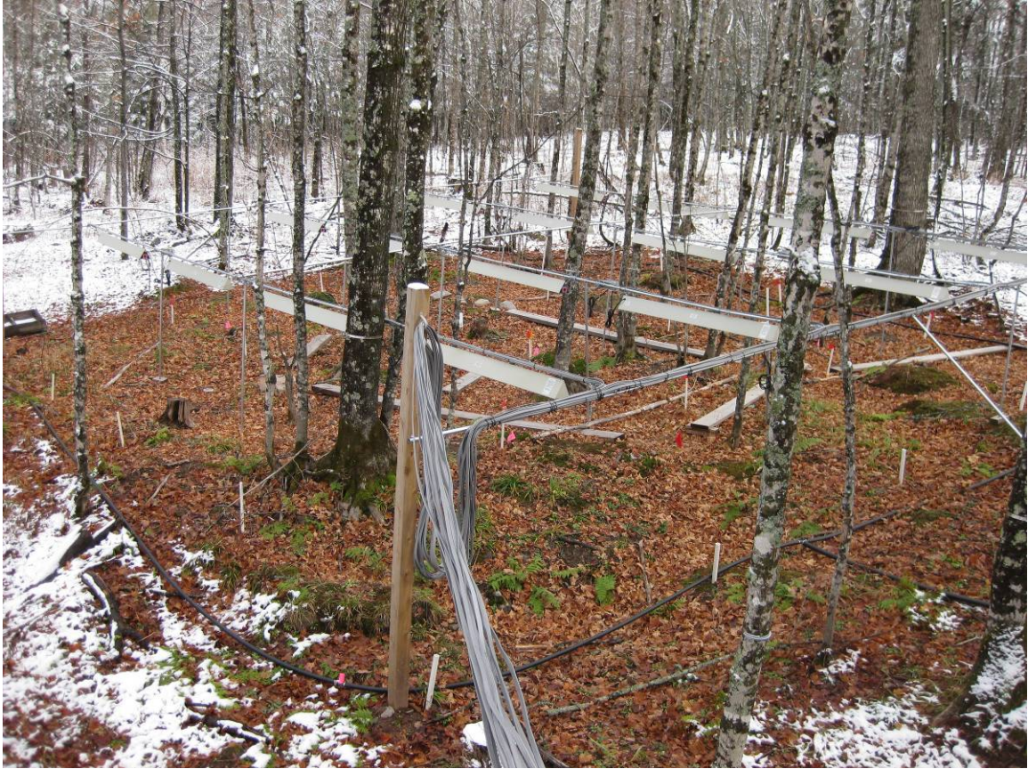
Figure 2.2. The heated footprint illustrated in snow reflects the complete dispersal of heat evenly across the 10 m by 10 m treatment plot. Note the heat extends beyond the 10 m by 10 m plot (Photo by M. Jarvi).
