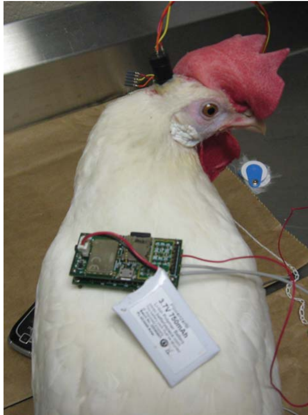
Figure 2.13: Chicken welfare experiment setup for EEG waveform acquisition.
