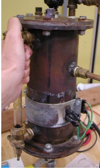
Figure 3.23: The evaporator without heat insulators.
