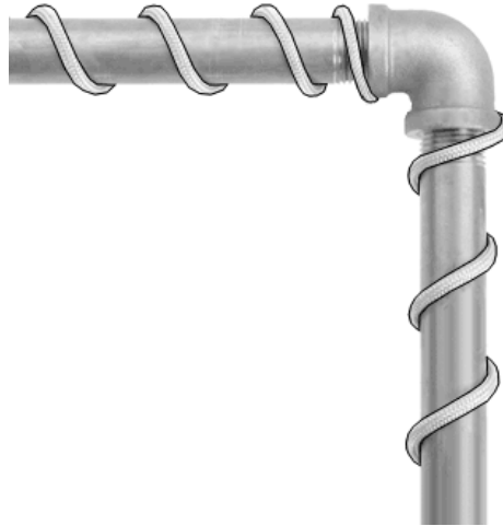
Figure 3.13: Typical rope heater used at the exit of the evaporator.
