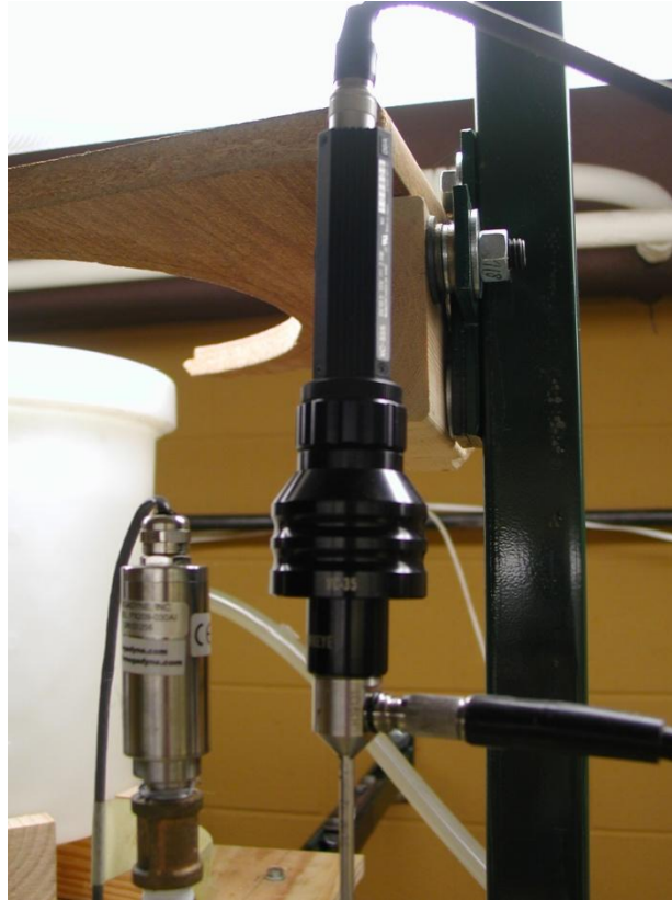
Figure 3.29: Borescope with video camera mounted on top of the test section.
