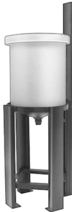
Figure 3.5: Water tank mounted at the highest point of the primary cooling loop.
