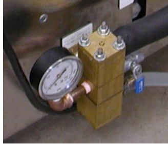
Figure 3.11: A picture of the customized three way valve.
