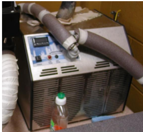
Figure 3.16: Picture of the Teca chiller installed in the secondary water loop.
