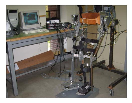
Figure (7 - 7) Testing system of ground reaction force for trailing leg
