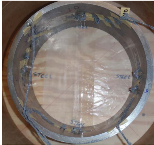
Figure 3.5: Complete strain gage installation
