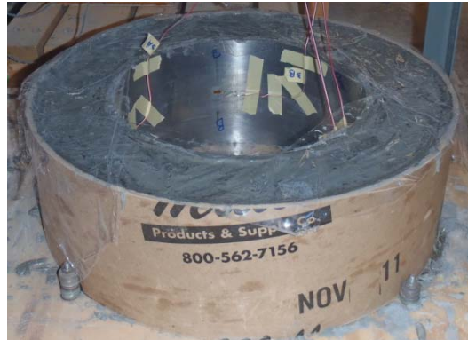
Figure 3.8: AASHTO PP34-99 cast specimen
