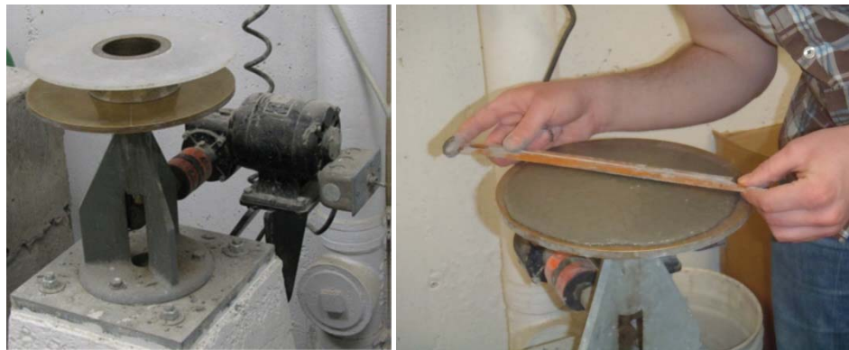
Figure 3.2: Flow test setup and spread measurement
