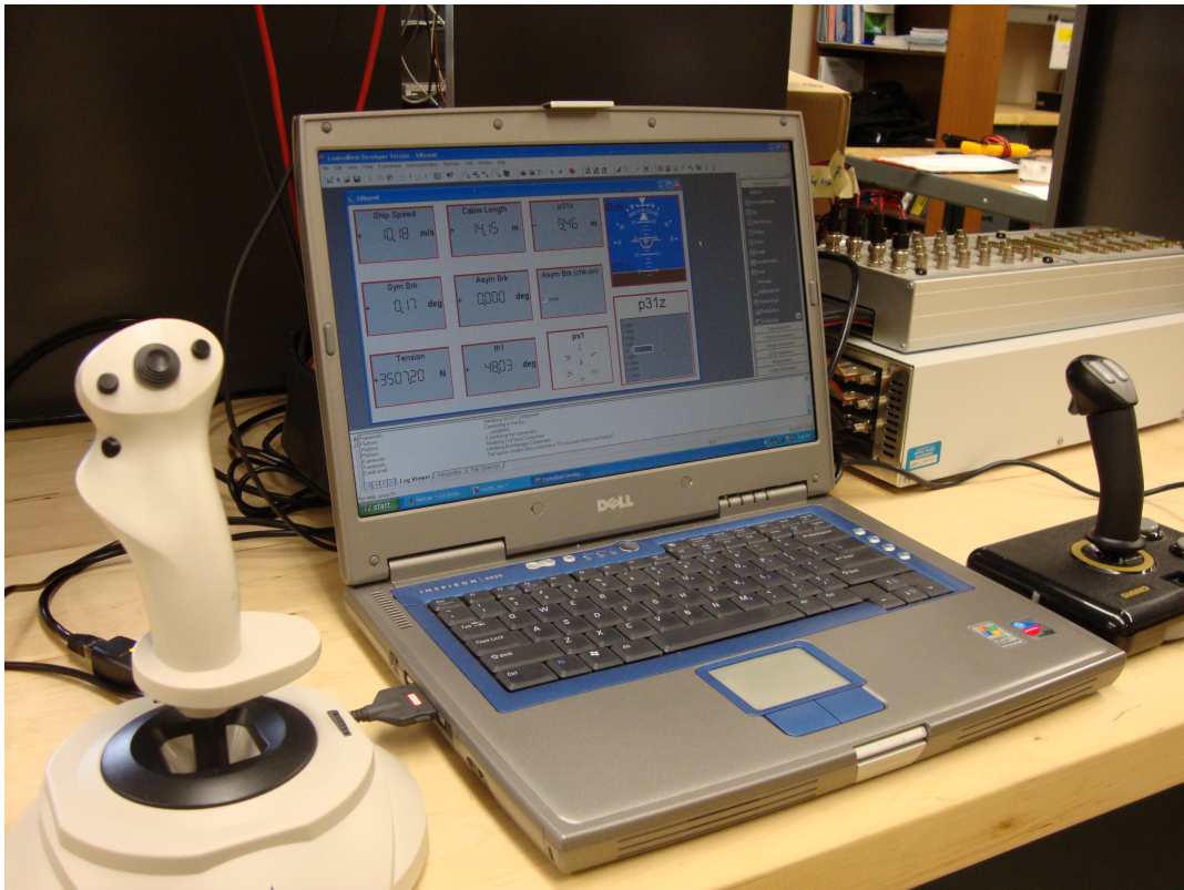
Figure 3.16. Operator-In-Loop simulation setup
