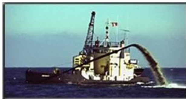
Figure 1.4: Sidecaster Dredge (USACE 2008) (Documentation can be found in Appendix E)
