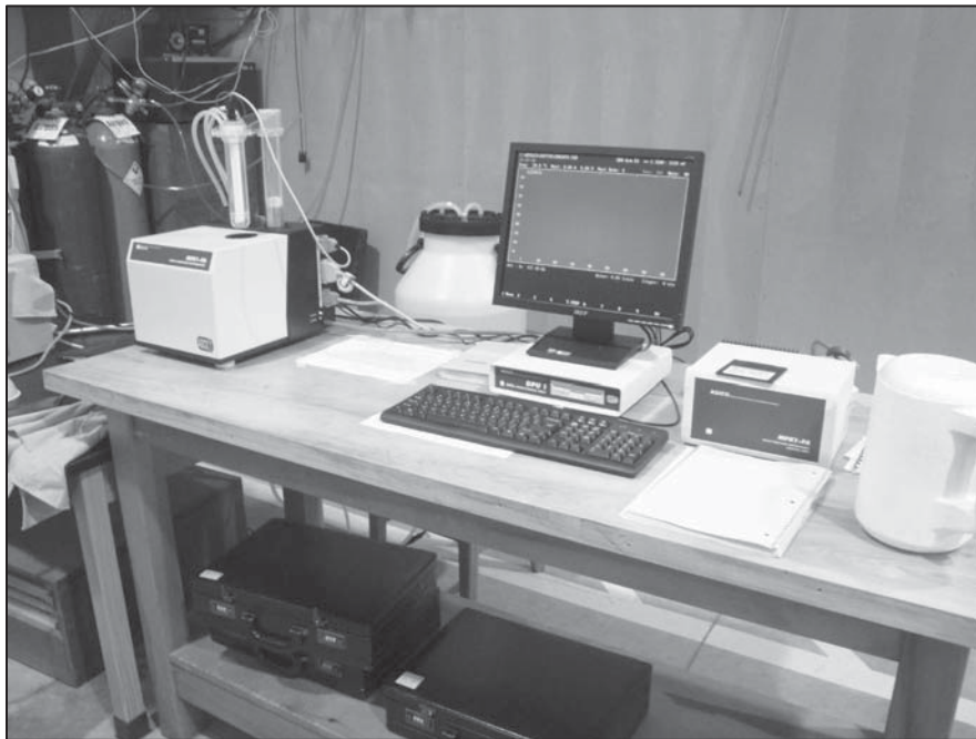
Figure 4.3: Photo of the Kappabridge instrument used during this study.
