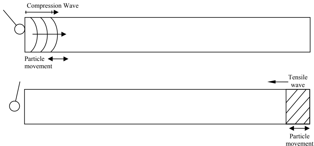
Figure 10. Travel of compression wave along log. The forward-moving wave impinges on the free end of the log, is reflected as a tensile wave, and begins to travel back down the log (Pellerin and Ross 2002).
