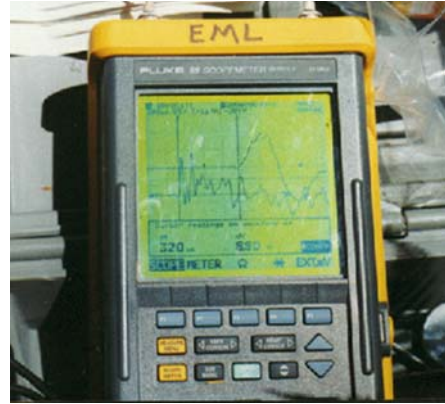
Figure 8. Start and stop signals from accelerometers shown on oscilloscope.
