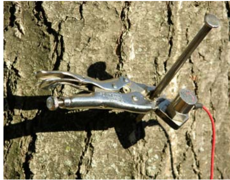
Figure 7. Accelerometer clamped onto a spike embedded into stem at 45° to grain.
