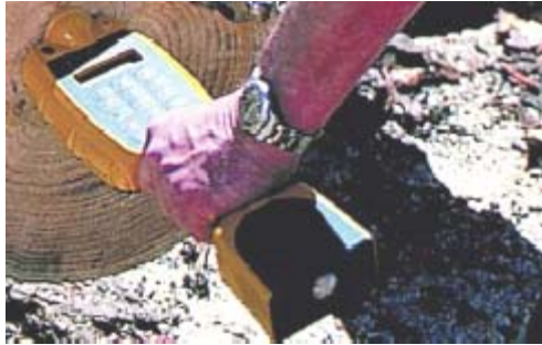
Figure 11. Log acoustic properties measured with a resonance stress wave technique using the Director HM200.
