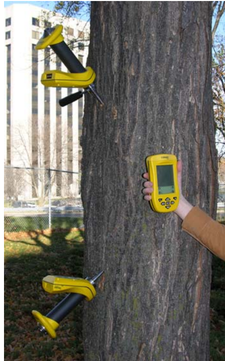
Figure 9. Setup of commercial tree assessment tool includes specially-designed probes and a PDA for wireless data collection.
