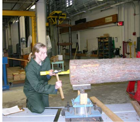
Figure 12. Determining acoustic properties of red pine logs with Director HM200 (fibre-gen, Auckland, New Zealand).
