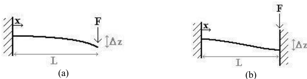
Figure 6.3: Beam-bending diagrams illustrating (a) the simple cantilever beam and (b) the double-clamped beam under a concentrated load, F , applied at x=L .
