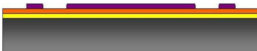
Figure 6.5(b): Device wafer following deposition and patterning of poly0 lower interconnect layer. Outer portions represent electrical traces while the center region reflects the ground plane below the structure.
