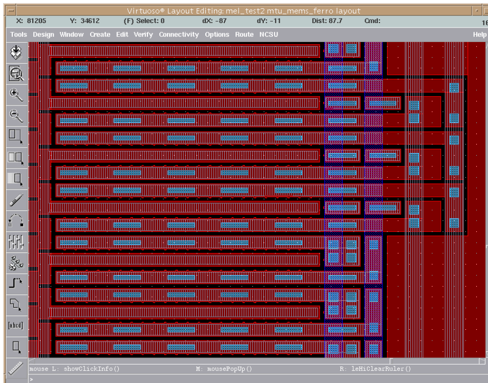
Figure 6.6(c): Close-up of sense electrode region showing dimensions of moving and stationary electrodes and surrounding gaps, vias, etch holes, and anti-stiction “bumps.”
