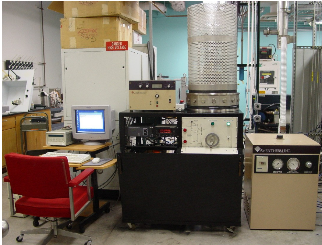
Figure 4.8: Full view of the BEAVIS test system showing the exterior layout. The system consisted of an induction power supply that operated a remote heat station within a vacuum chamber. It was constructed for the purpose of optimizing the induction heating of thin ferromagnetic films.
