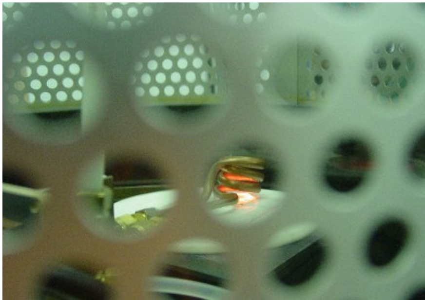
Figure 4.22: Photograph showing a sample being heated using an early configuration of BEAVIS. This sample measured 4\text{cm}^2 in area and 2.5\mu\text{m} in thickness. It was being heated at approximately 1.5kW to around 1000^\circ\text{C} . Glowing was typically first observed at around 600^\circ\text{C} and grew in intensity with increasing temperature.
