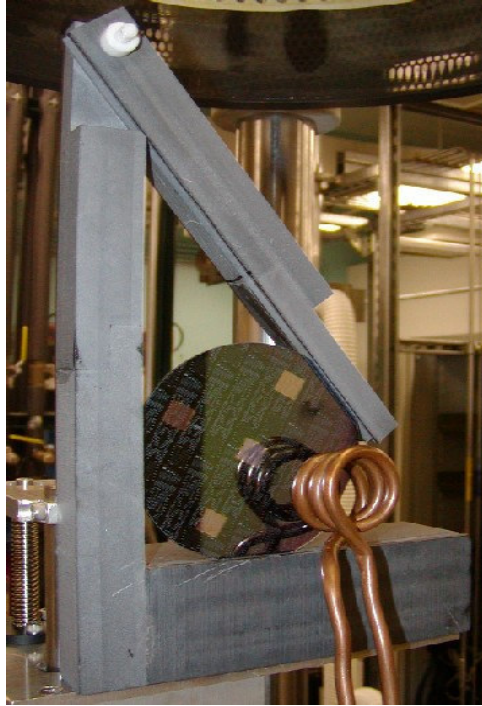
Figure 4.12: Alumina silicate (ceramic) substrate holder designed to secure the wafer vertically in front of the coil without placing restrictions on wafer diameter or heat sinking capability. Shown here is a 4” silicon wafer with 1\text{cm}^2 FeCo films in an attempt to heat groups of polysilicon test structures.
