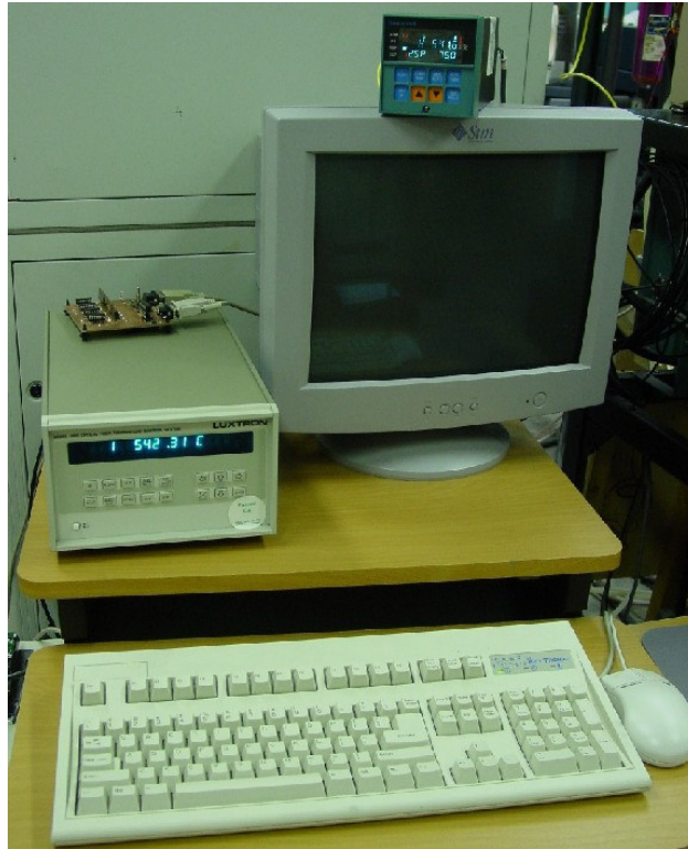
Figure 4.17: Illustration of the pyrometry calibration procedure in which the thermocouple readout was displayed on the green-colored system above the computer monitor while the pyrometry readout was displayed on the tan-colored system to the left of the monitor. The pyrometer had just been supplied with the known reference temperature.
