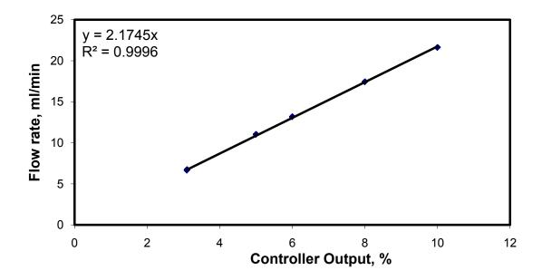
Figure (2-3): Oxygen Mass Flow Controller Calibration Results
