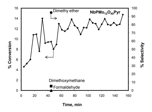
Figure (3-9) - Conversion and selectivity of NbPMo<sub>12</sub>O<sub>40</sub>Pyr catalyst as a function of time. The reaction was carried out at 260°C and with 0.01g of catalyst and a total flow-rate of 157.3 (ml/min) (He/O<sub>2</sub>/MeOH =115.2/20.44/27.34 ml/min).
