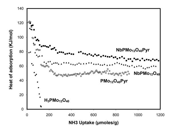
Figure (3-1) -  $NH_3$  uptake and heat of adsorption of the catalysts showing the active sites. All the catalysts activated at 420°C
