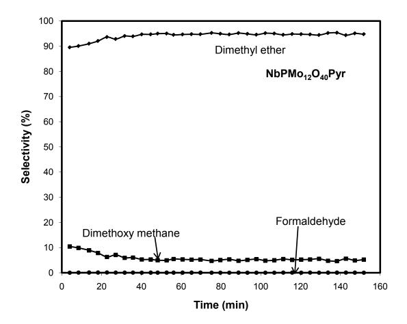
Figure (3-10) - Selectivity of all products as a function of time of NbPMo<sub>12</sub>O<sub>40</sub>Pyr catalyst. The reaction was carried out at 260°C and with 0.01g of catalyst and a total flow-rate of 157.3 (ml/min) (He/O<sub>2</sub>/MeOH =115.2/20.44/27.34 ml/min).
