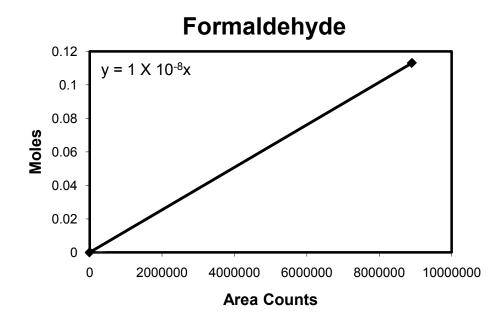
Figure (2-5): Calibration Curve for Formaldehyde (GC/MS)
