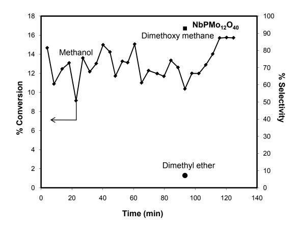
Figure (3-5) - Conversion and selectivity of NbPMo<sub>12</sub>O<sub>40</sub> catalyst as a function of time. The reaction was carried out at 260°C and with 0.04g of catalyst and a total flowrate of 108.2 (ml/min) (He/O<sub>2</sub>/MeOH = 76.5/13.5/18.2 ml/min).
