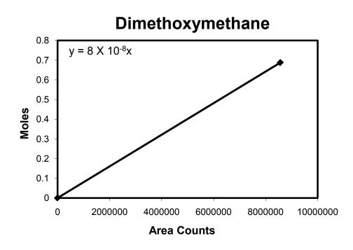
Figure (2-6): Calibration Curve for Dimethoxymethane (GC/MS)
