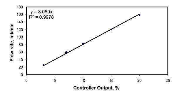
Figure (2-2): Helium Mass Flow Controller Calibration Results
