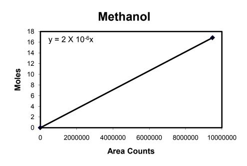
Figure (2-4): Calibration Curve for Methanol (GC/MS)
