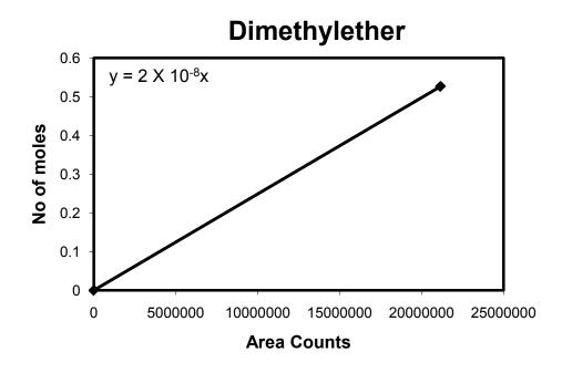
Figure (2-7): Calibration Curve for Dimethyl Ether (GC/MS)
