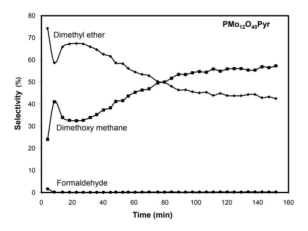
Figure (3-8) - Selectivity of all products as a function of time of PMo<sub>12</sub>O<sub>40</sub>Pyr catalyst. The reaction was carried out at 260°C and with 0.04g of catalyst and a total flowrate of  $108.2 \text{ (ml/min)} (\text{He/O}_2/\text{MeOH} = 76.5/13.5/18.2 \text{ ml/min}).$
