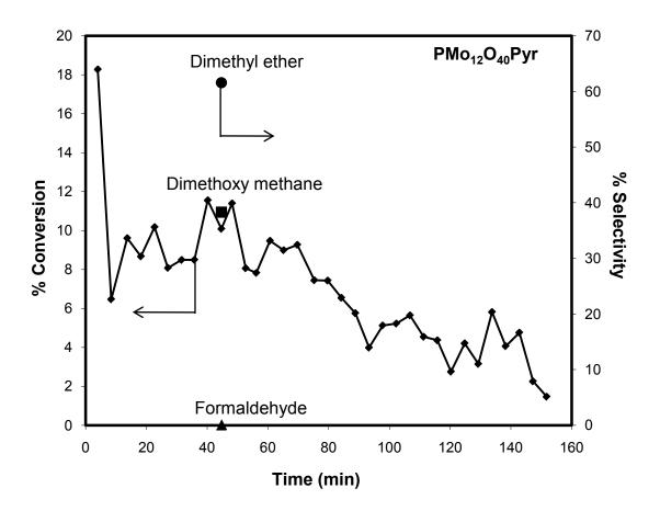
Figure (3-7) - Conversion and selectivity of  $PMo_{12}O_{40}Pyr$  catalyst as a function of time. The reaction was carried out at 260°C and with 0.04g of catalyst and a total flowrate of 108.2 (ml/min) (He/O<sub>2</sub>/MeOH =76.5/13.5/18.2 ml/min).
