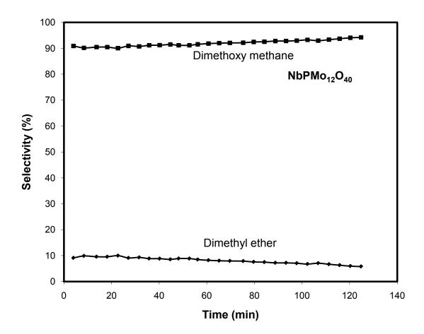
Figure (3-6) - Selectivity of all products as a function of time of NbPMo<sub>12</sub>O<sub>40</sub> catalyst. The reaction was carried out at 260°C and with 0.04g of catalyst and a total flowrate of 108.2 (ml/min) (He/O<sub>2</sub>/MeOH =76.5/13.5/18.2 ml/min).
