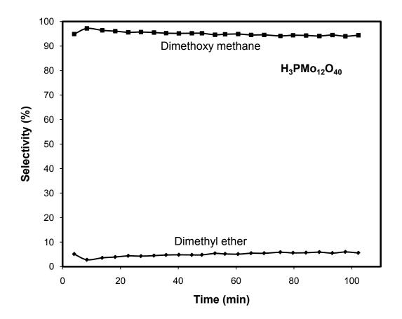
Figure (3-4) - Selectivity of all products as a function of time of  $H_3PMo_{12}O_{40}$  catalyst. The reaction was carried out at 260°C and with 0.02g of catalyst and a total flowrate of 96.2 (ml/min) (He/O<sub>2</sub>/MeOH =67.69/11.95/16.2 ml/min)
