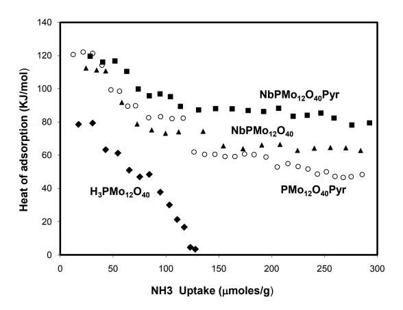
Figure (3-2) -  $NH_3$  uptake and heat of adsorption of the catalysts showing the active sites. All the catalysts activated at 420°C
