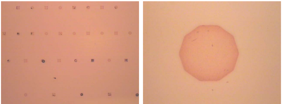
Figure 26: Optical microscope images of oriented PM film patterns (OD = 3.25) electrodeposited onto a gold coated silicon wafer patterned by photolithography. (left = 5X, right = 100X)
