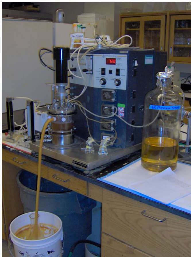
Figure 3: New Brunswick Scientific Bioflo III Continuous/Batch Fermentor growing H. salinarum .
