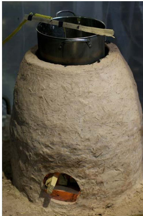
Figure 3-2 Shielded fire stove during a Water Boiling Test for 1 L of water in a 30 cm diameter pot
