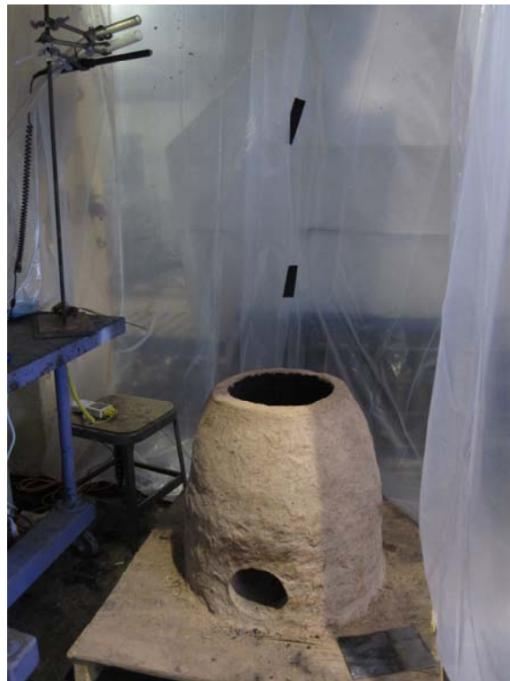
Figure 3-5 Emissions sampling set up during stove testing; instrument sampling inlets were positioned 1 m above pot atop stove
