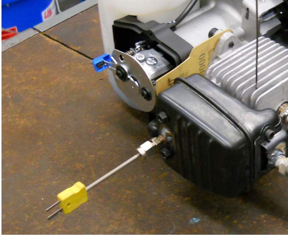
Figure 3.4: Exhaust gas thermocouple installation
