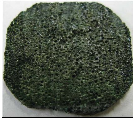
Fig. 3.3. Example of 45 min deposited electrode (photo by M. B. Chye).
