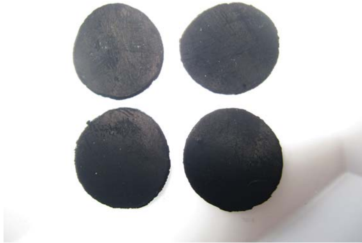
Fig. 3.5. Carbon black electrodes (3 wt% PTFE/CB and 97% Ketjenblack, EC-600JD) (photo by the author).
