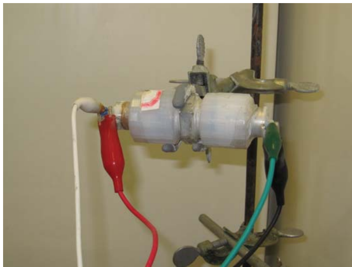
Fig. 3.6. Swagelok cell connected for charge-discharge cycling (photo by the author).
