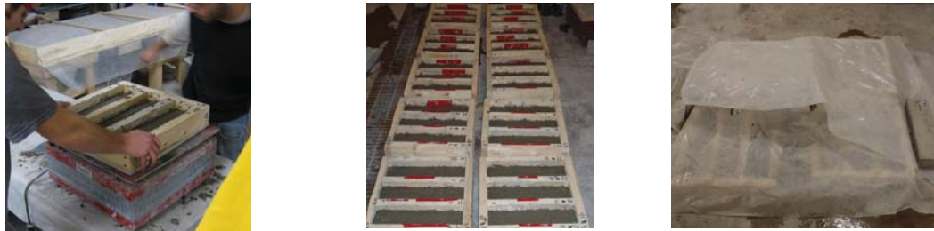
(a) Vibration for 5-10 seconds was applied once NSC was placed into moulds. (b) Moulds before covering them with plastic. (c) Moist cure: cylinders with water were placed before covering with plastic.
