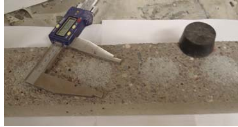
(a) Sample macro texture depth of concrete beams
