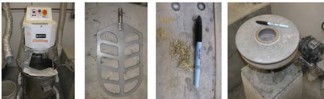
(a) Doyon BFT-060 planetary mixer. (b) Mixer paddle. (c) Steel fibers. (d) Equipment for the Slump test.
