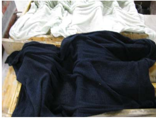
(a) Concrete substrate under water for 24 hours before placing the overlay material
