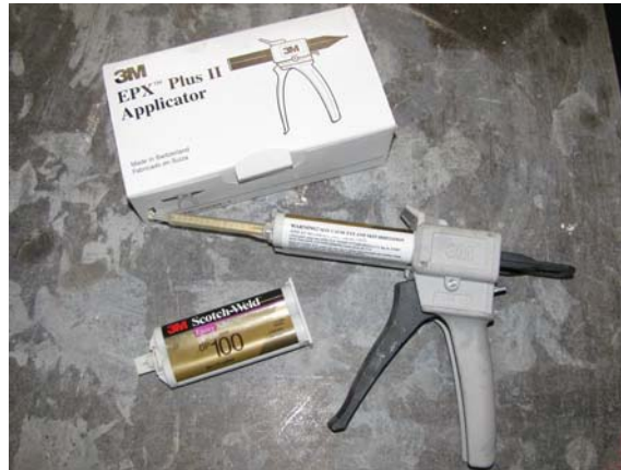
(b) Adhesive to glue the steel disk to the overlay surface
