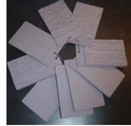
(b) Concrete Surface Preparation index
