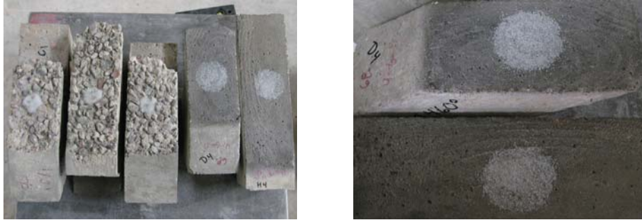
Sample macro texture depth of concrete substrates for the slant shear test.
