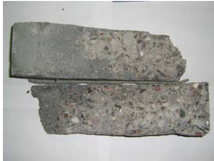
(c) B-C: Mixture failure of bond and concrete.
