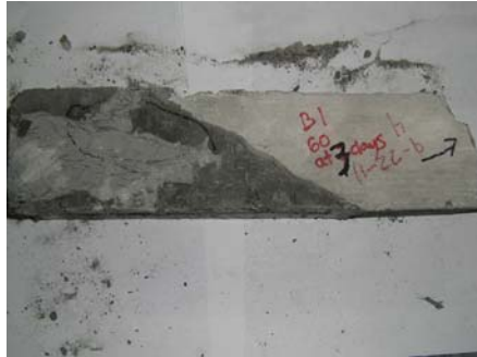
(e) Cohes: Cohesive failure.
