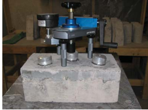
(b) The set up for the pull off test
