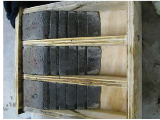
(b) Concrete substrate under water for 24 hours before placing the overlay material
