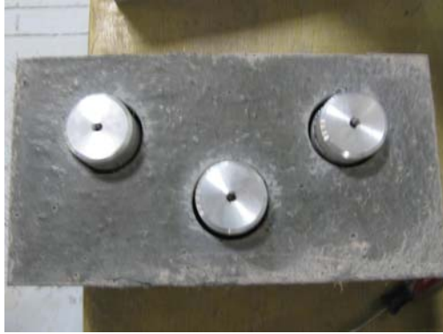
(a) Steel disks glued to the UHPC surface
