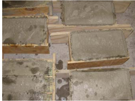
(a) Concrete substrates for the pull off test before demoulding.
