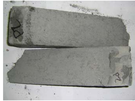
(b) B(UHPC): Bond due to UHPC failure.
