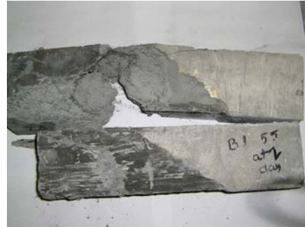
(f) UHPC: UHPC failure.
