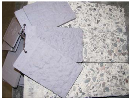
Comparing different ICRI profiles for the rough surface.
