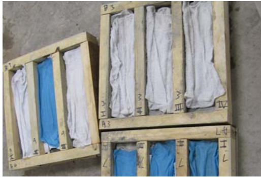
(c) Wet cloths covering the concrete substrate
