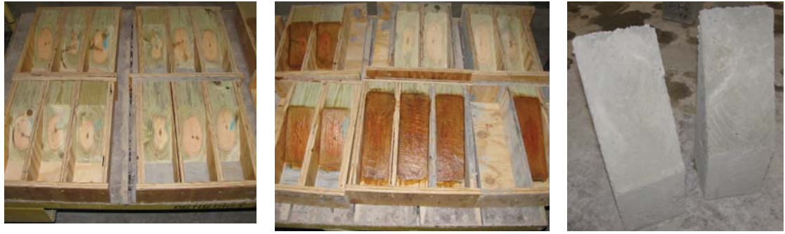
(a) Molds to cast slant shear specimens. (b) Molds after applying a concrete surface retarder to obtain a rough surface. (c) NSC substrate for slant shear samples after demolding.
