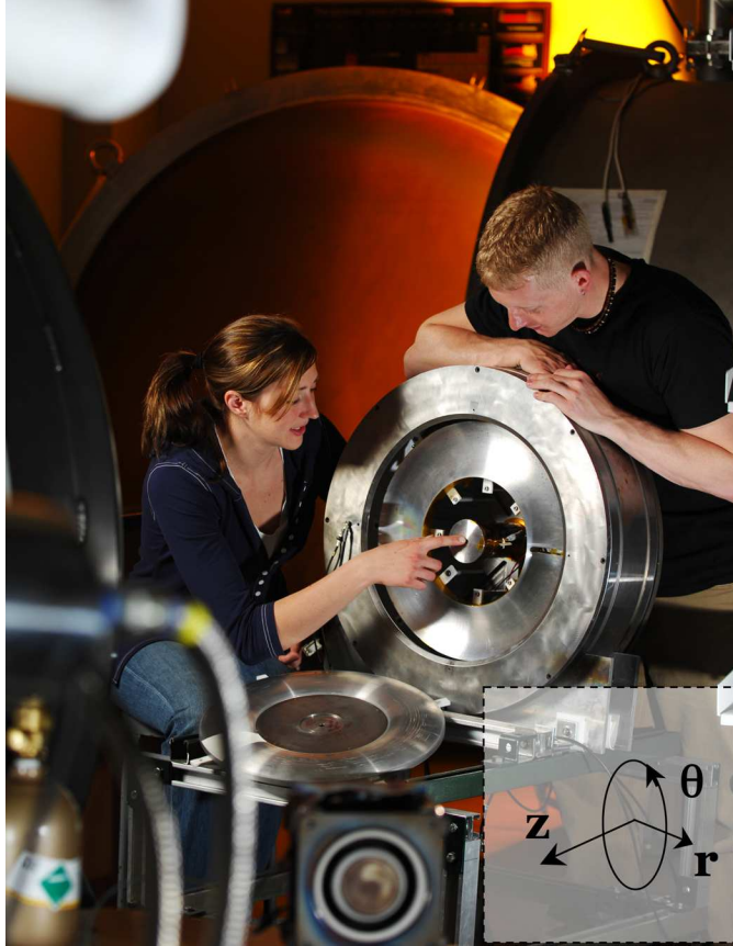
Figure 4.1: Photograph of the Hall Electron Mobility Gage (cathode electrode and center front plate have been removed and are shown in the photo laying in front of the apparatus). Orientation shown at the bottom right of the figure. (Photo courtesy of Ref. [4])
