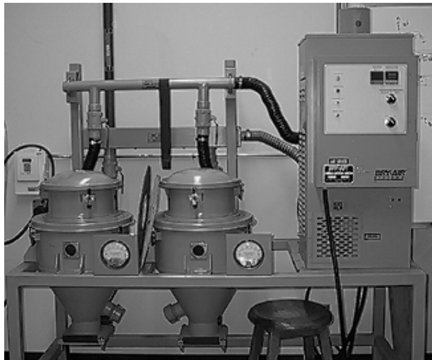
Figure 4.1-1: Bry Air Dryer System
