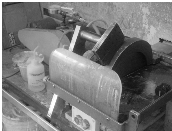
Figure 4.2-8: Image of Cut Off Saw Used to Cut Epoxy Puck into Thin Sections
