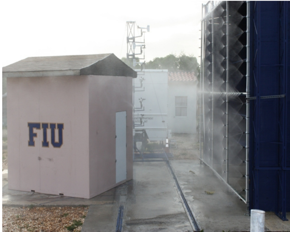
Figure 3.2: Wind Driven Rain Testing at FIU Wall of Wind
