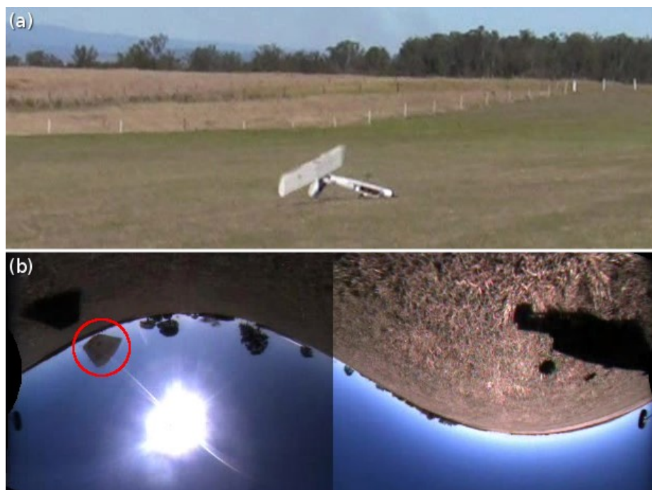
Figure 9.1: Failure case for aircraft guidance: detachment of wing from aircraft body. The moment of impact was captured by (a) an external camera and (b) the iEye vision system on board the aircraft. Extreme attitude and proximity to the ground in conjunction with the wing (red circle) visibly separated from the aircraft should have alerted the on-board guidance system to an ‘abnormal control situation’. Unfortunately the control system was not optimally tuned to cope with such eventualities.
