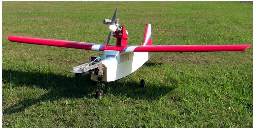
Figure 3.12: The aircraft used for collision avoidance and terrain following flight tests with the stereo vision system mounted on the nose.
