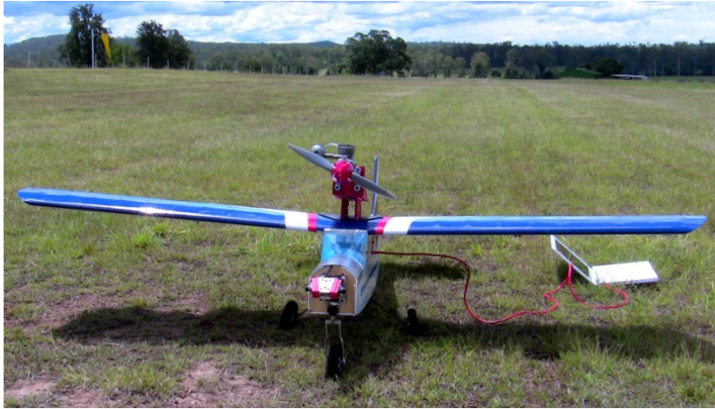
Figure 6.7: The aircraft used for the flight tests discussed in Part II with the iEye vision system mounted on the nose.
