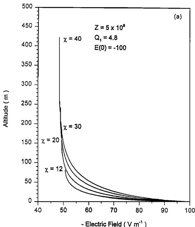
Figure 4. Vertical profiles of (a) electric field (b) small-ion concentration, and (c) charged aerosol concentration when  $\chi = 12, 20, 30,$  and  $40 \text{ m}^2 \text{ s}^{-1}$ ,  $Q_1 = 4.8$ ,  $Z = 5 \times 10^8 \text{ m}^{-3}$  and  $E(0) = -100 \text{ V m}^{-1}$ .
