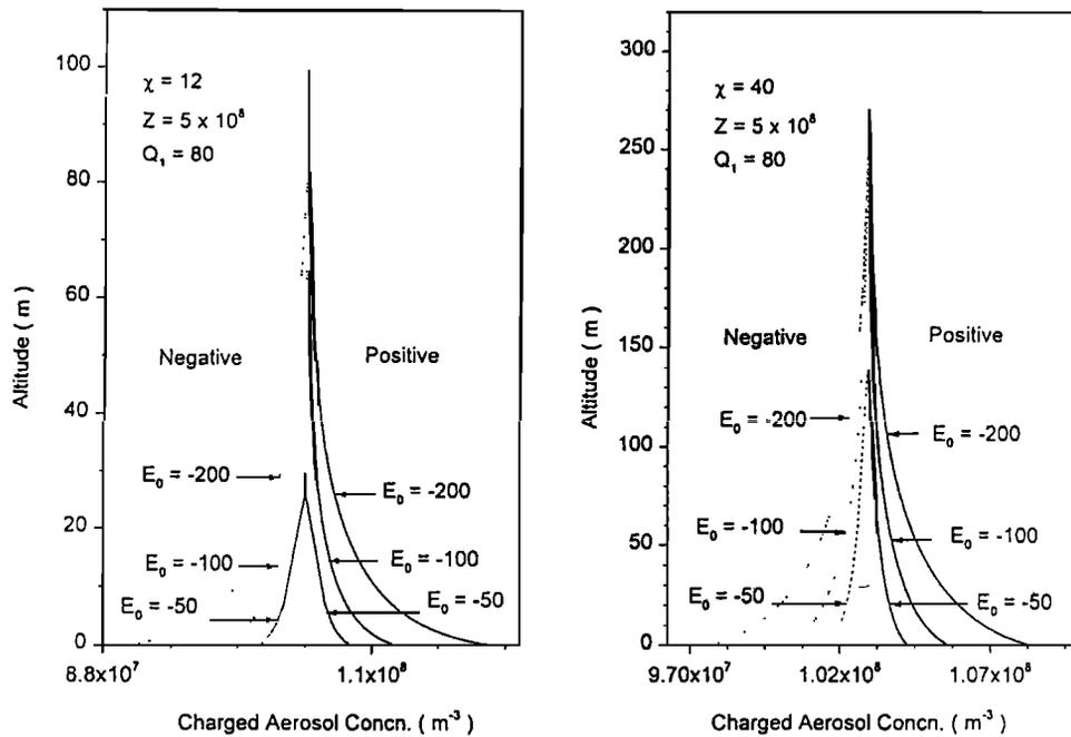
Figure 3. Vertical profiles of charged aerosol concentration when  $\chi = 12$  and  $40 \text{ m}^2 \text{ s}^{-1}$ ,  $Q_1 = 80$ ,  $Z = 5 \times 10^8 \text{ m}^{-3}$ , and  $E(0) = -50, -100$  and  $-200 \text{ V m}^{-1}$ .
