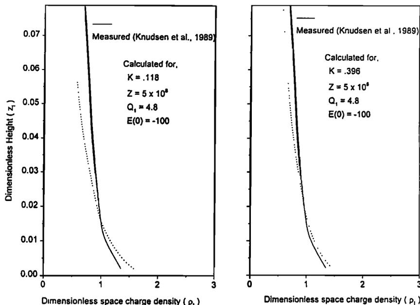
Figure 6. Comparison of calculated results when  $\chi = 12, 40 \text{ m}^2 \text{ s}^{-1}$  ( $K(z) = 0.118, 0.396 \text{ m}^2 \text{ s}^{-1}$ ),  $Q_1 = 4.8$ ,  $E(0) = -100 \text{ V m}^{-1}$ , and  $Z = 5 \times 10^8 \text{ m}^{-3}$  with experimental results by *Knudsen et al.* [1989] for the variation of dimensionless space charge density with dimensionless height.
