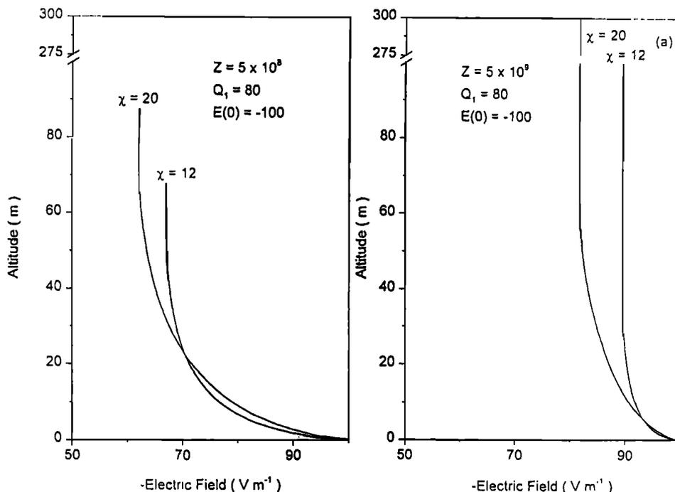
**Figure 2.** Vertical profiles of (a) electric field, (b) small-ion concentration, and (c) charged aerosol concentration when  $\chi = 12$  and  $20 \text{ m}^2 \text{ s}^{-1}$ ,  $Q_1 = 80$ ,  $Z = 5 \times 10^8$  and  $5 \times 10^9 \text{ m}^{-3}$  and  $E(0) = -100 \text{ V m}^{-1}$ .
