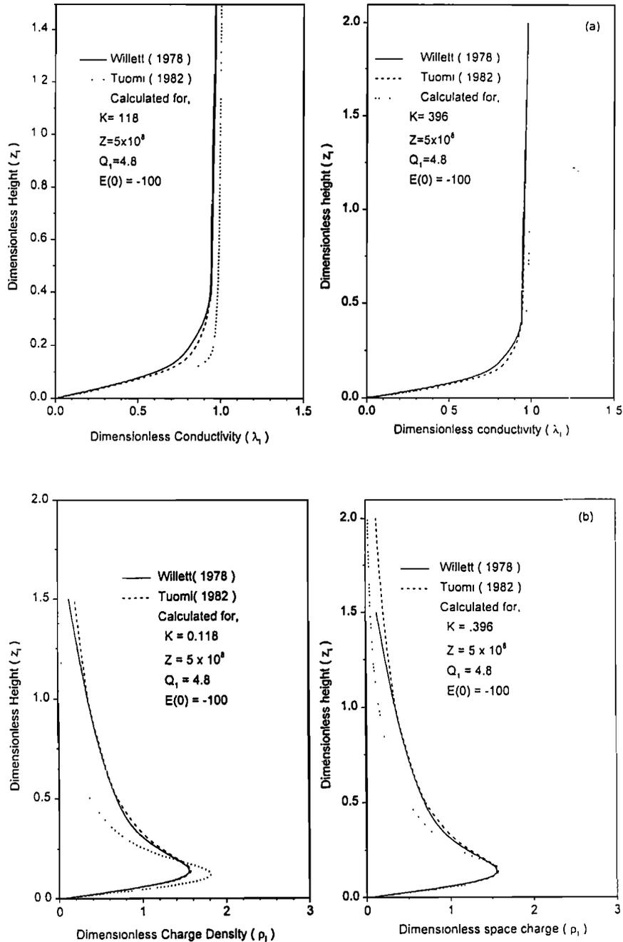
**Figure 5.** Comparison of calculated results of variation of (a) dimensionless conductivity and (b) dimensionless space charge density with dimensionless height when  $\chi = 12$  and  $40 \text{ m}^2 \text{ s}^{-1}$  ( $K(z) = 0.118, 0.396 \text{ m}^2 \text{ s}^{-1}$ ),  $Q_1 = 4.8$ ,  $E(0) = -100 \text{ V m}^{-1}$ , and  $Z = 5 \times 10^8 \text{ m}^{-3}$  with previous theoretical results by *Willett [1978]* and *Tuomi [1982]*.
