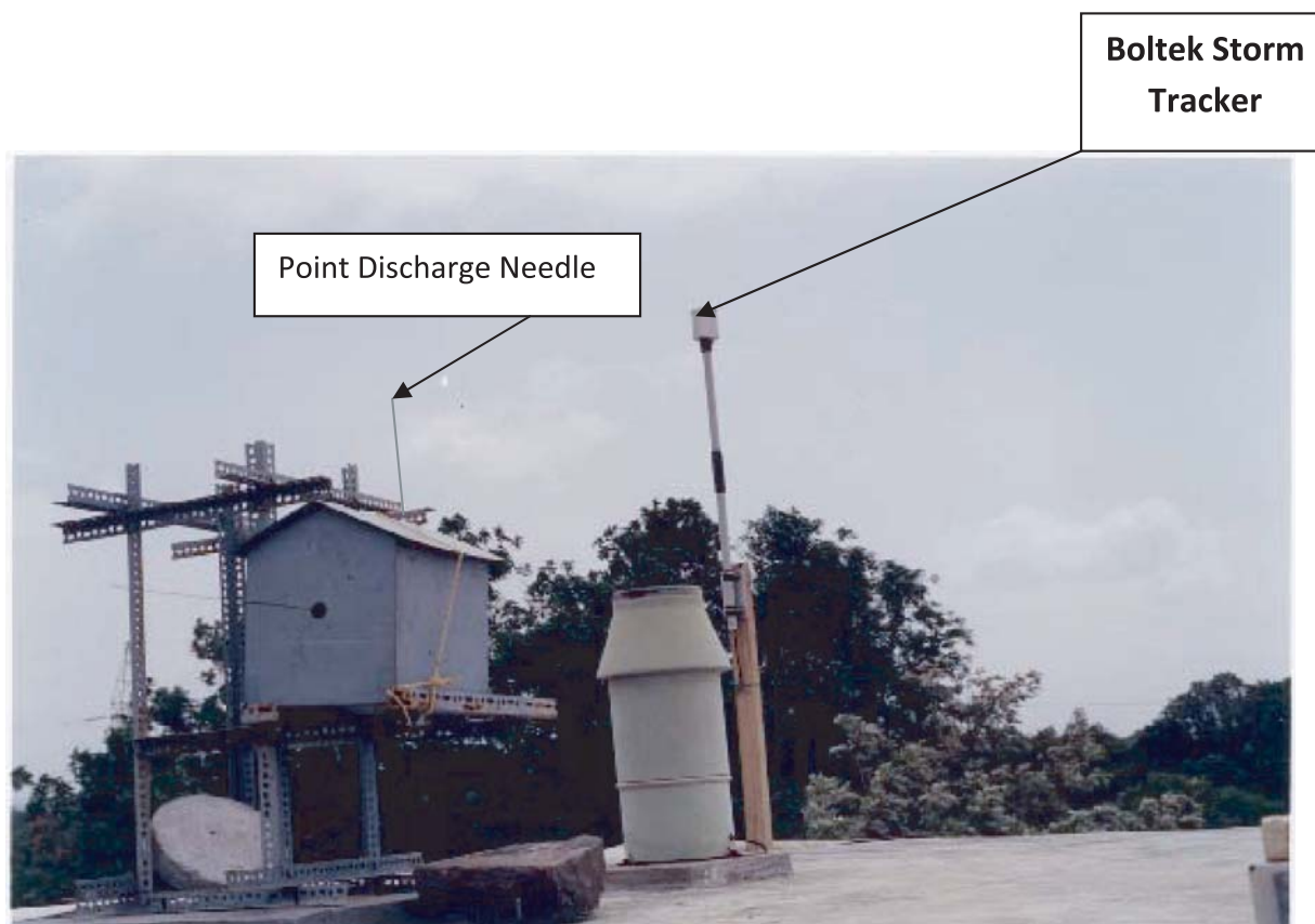
Fig. 2. System of Boltek Storm Tracker installed on the terrace of IITM, Pune
