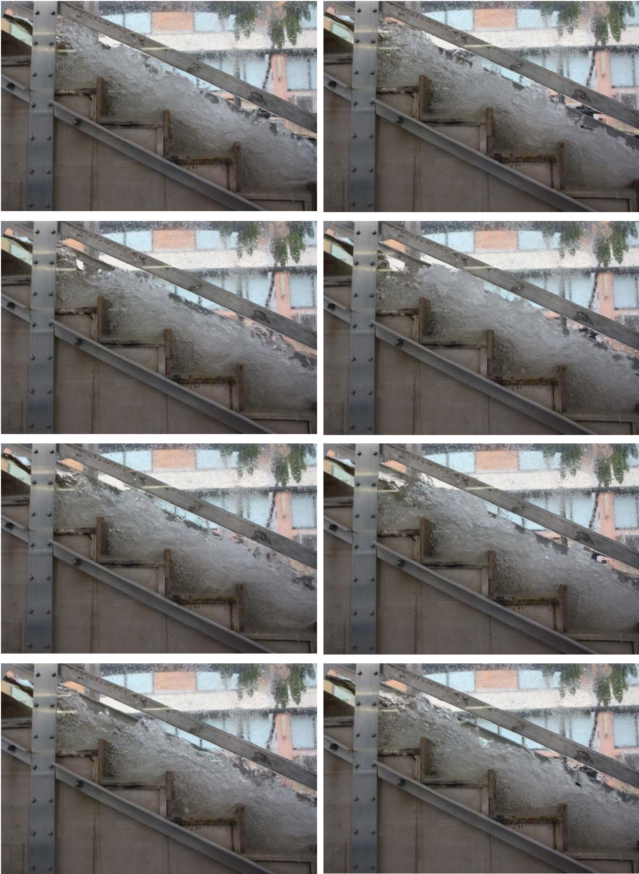
Fig. A-11 – Small instabilities in the transition flow regime on the pooled stepped spillway ( \theta = 26.6^\circ . w = 3.1 cm): d_c/h = 0.88 , Q = 0.043 m 3 /s, Re = 3.3 \times 10^5 (order from top left to bottom right)
