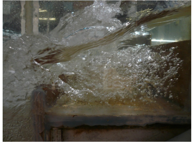
(B) d_c/h = 0.66 , Q = 0.028 m 3 /s, Re = 2.1 \times 10^5
