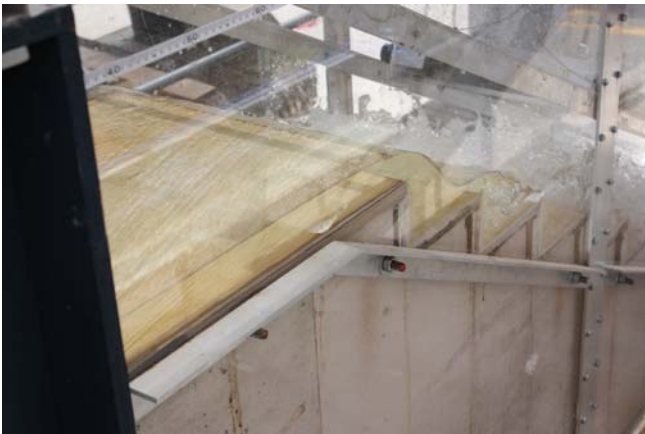
Fig. A-6 – Transition flow regime on the flat stepped spillway ( \theta = 26.6^\circ )
