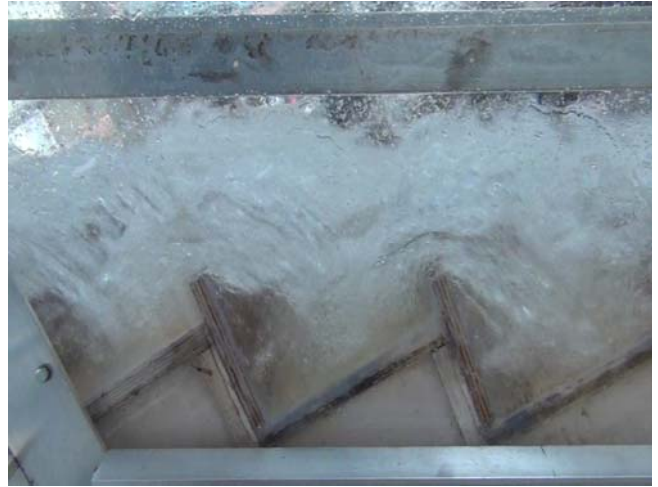
Fig. A-15 –Nappe flows (pooled step side) and transition flows (flat side) on the stepped spillway with in-line configuration of flat and pooled ( w = 3.1 cm) steps ( \theta = 26.6^\circ ) for 0.46 \leq d_c/h \leq 0.55 (A) d_c/h = 0.46 , Q = 0.016\text{m}^3/\text{s} , Re = 1.2 \times 10^5 (B) d_c/h = 0.46 , Q = 0.016\text{m}^3/\text{s} , Re = 1.2 \times 10^5
