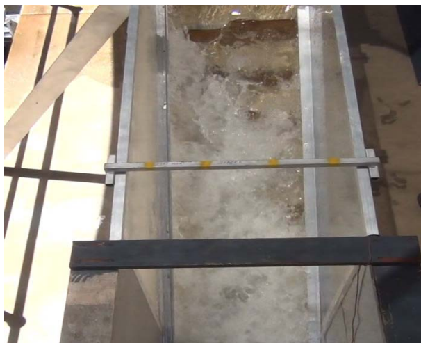
(C) Shockwaves, d_c/h = 0.86 , Q = 0.041 \text{ m}^3/\text{s} , Re = 3.1 \times 10^5
