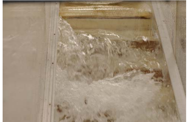
Fig. A-19 – Transition and skimming flow regime on the stepped spillway with in-line configuration of flat and pooled ( w = 3.1 cm) steps ( \theta = 26.6^\circ )
