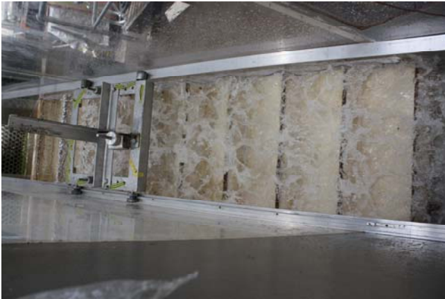
Fig. A-5 – Nappe flow regime on the flat stepped spillway ( \theta = 26.6^\circ )
