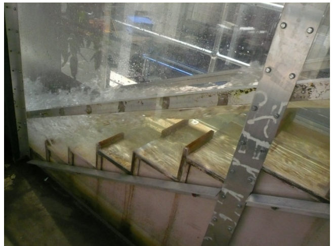
(F) d_c/h = 1.80 , Q = 0.124 \text{ m}^3/\text{s} , Re = 9.5 \times 10^5
