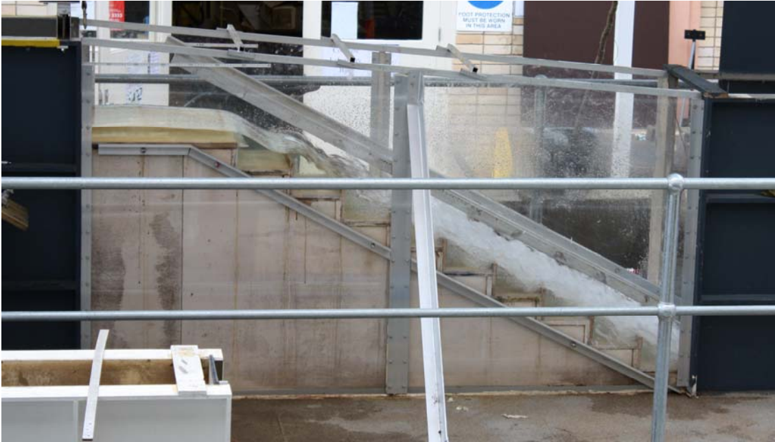
Fig. 2-1 – Experimental test section in the present study: pooled stepped spillway configuration - Flow conditions: d_c/h = 0.53 , Q = 0.020 \text{ m}^3/\text{s} , Re = 1.54 \times 10^5 (Note the broad-crested weir upstream of the first step edge) - Flow direction from left to right
