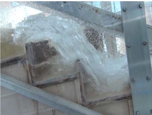
(C) d_c/h = 0.46 , Q = 0.016\text{m}^3/\text{s} , Re = 1.2 \times 10^5
