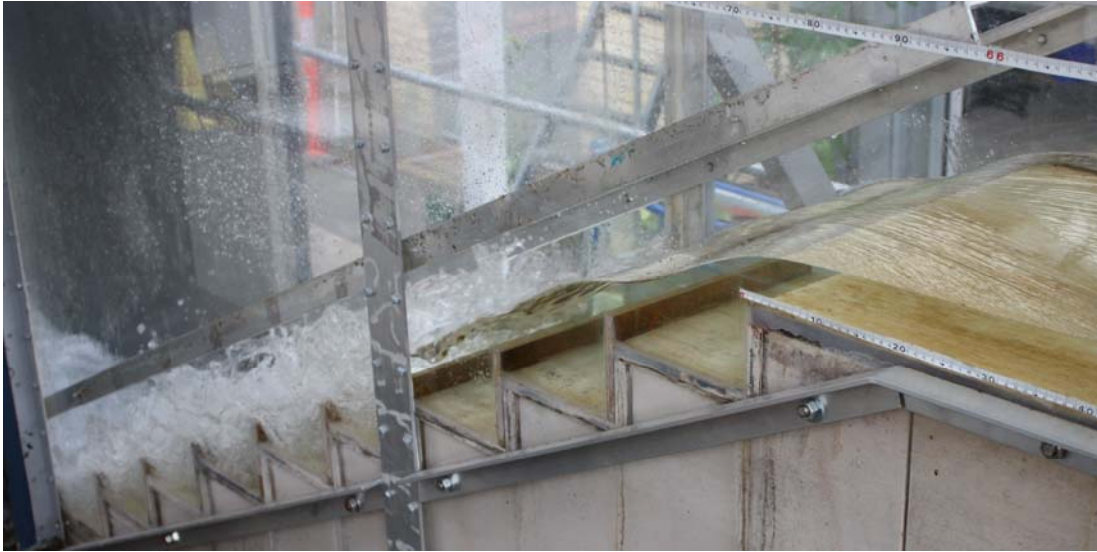
Fig. 3-4 – Transition flow regime on pooled stepped spillway: d_0/h = 0.71 , Q = 0.031 \text{ m}^3/\text{s} , Re = 2.4 \times 10^5
