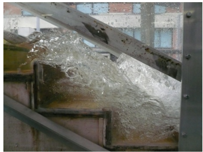
(D) Standing sidewall waves, d_c/h = 0.59 , Q = 0.023 \text{ m}^3/\text{s} , Re = 1.8 \times 10^5
