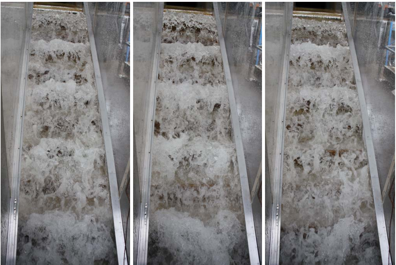
Fig. E-3 – Pulsating flow on the pooled stepped spillway ( d_c/h = 0.4 , Q = 0.013 \text{ m}^3/\text{s} , Re = 1.0 \times 10^5 ) - Chronological order from left to right
