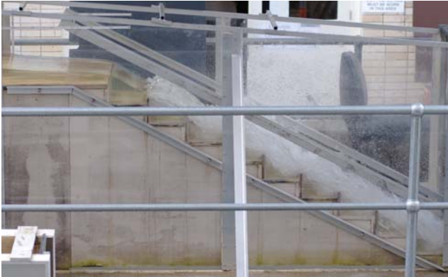
Fig. A-19 – Transition and skimming flow regime on the stepped spillway with in-line configuration of flat and pooled ( w = 3.1 cm) steps ( \theta = 26.6^\circ )
