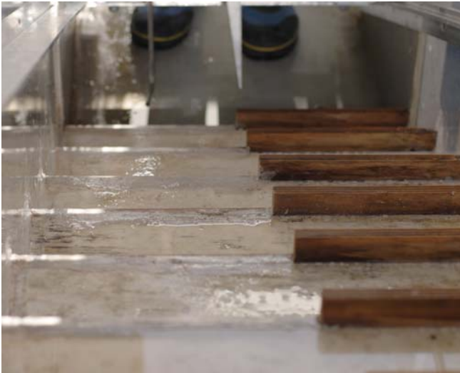
(C) Stepped spillway with in-line configuration of flat and pooled steps
