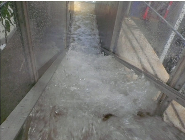
(C) d_c/h = 0.74 , Q = 0.033 m 3 /s, Re = 2.5 \times 10^5
