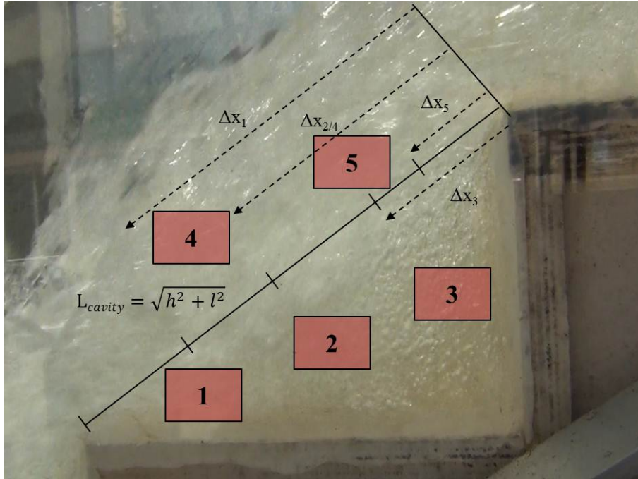
Fig B-3 - Recording positions for the cavity ejection video analysis on the flat and pooled stepped spillways ( \theta = 26.6^\circ )
