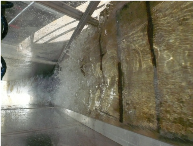
(E) d_c/h = 1.80 , Q = 0.124 \text{ m}^3/\text{s} , Re = 9.5 \times 10^5
