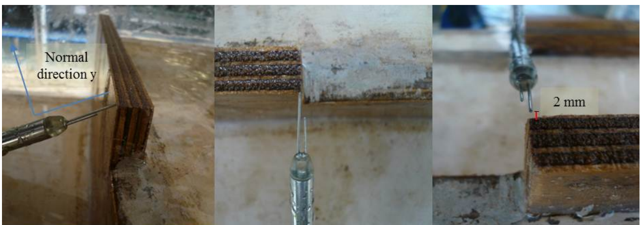
Fig. 5-2 – Position of double-tip conductivity probe ( \varnothing = 0.25 mm) on channel centreline ( z/W = 0.5 ) for the stepped spillways with in-line and staggered configurations of flat and pooled steps ( \theta = 26.6^\circ )
