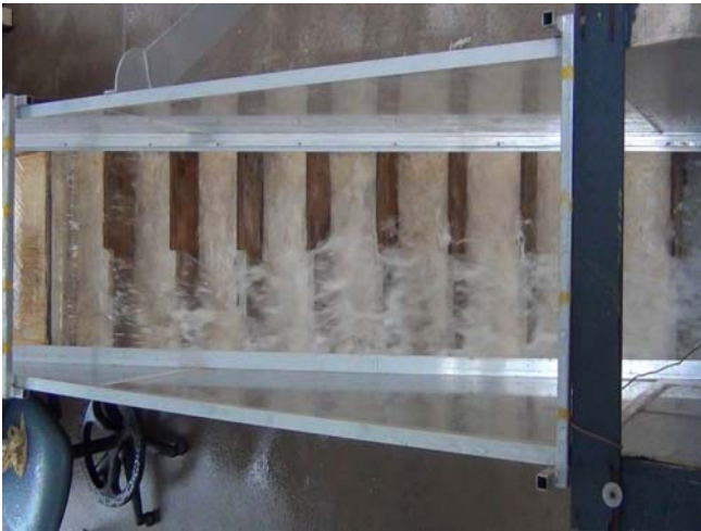
Fig. A-13 – Nappe flow regime on the stepped spillway with in-line configuration of flat and pooled (w = 3.1 cm) steps ( \theta = 26.6^\circ )
