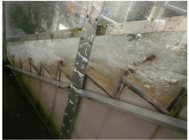
(B) d_c/h = 0.59 , Q = 0.023\text{m}^3/\text{s} , Re = 1.8 \times 10^5
