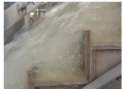
(B3) Distribution of air packet in cavity
