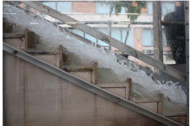
Fig. A-10 – Transition flow regime on the pooled stepped spillway ( \theta = 26.6^\circ , w = 3.1 cm)
