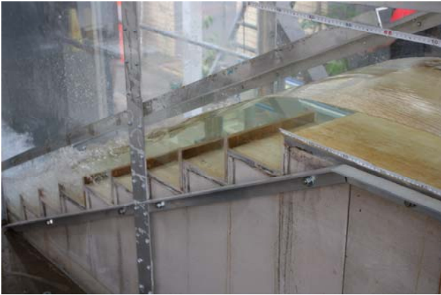
Fig. A-12 – Skimming flow regime on the pooled stepped spillway ( \theta = 26.6^\circ , w = 3.1 cm)
