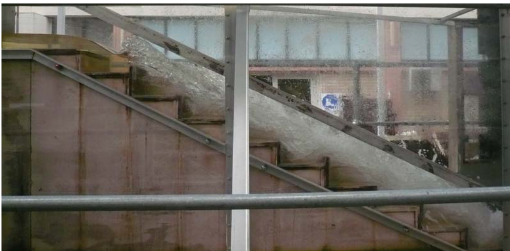
Fig. 3-12 – Transition flow regime on the stepped spillway with staggered configuration of flat and pooled steps ( \theta = 26.6^\circ ): d_c/h = 0.70 , Q = 0.030 \text{ m}^3/\text{s} , Re = 2.30 \times 10^5
