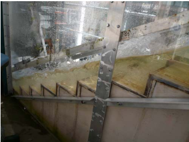
(C) d_c/h = 1.15 , Q = 0.063 m 3 /s, Re = 4.9 \times 10^5
