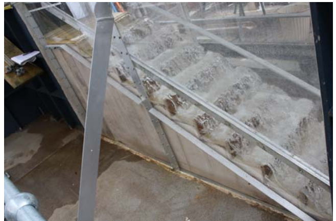
Fig. A-8 – Nappe flow regime on the pooled stepped spillway ( \theta = 26.6^\circ . w = 3.1 cm)
