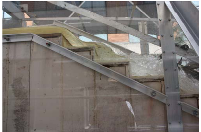
Fig. A-6 – Transition flow regime on the flat stepped spillway ( \theta = 26.6^\circ )
