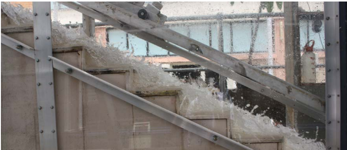
Fig. 3-1 – Air-water flow pattern on flat stepped spillway ( \theta = 26.6^\circ )
