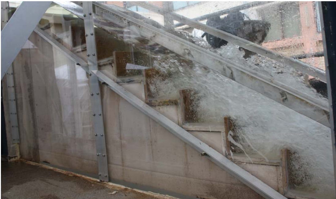
Fig. 3-5 – Skimming flow regime on pooled stepped spillway: d_0/h = 1.27 , Q = 0.074 \text{ m}^3/\text{s} , Re = 5.6 \times 10^5
