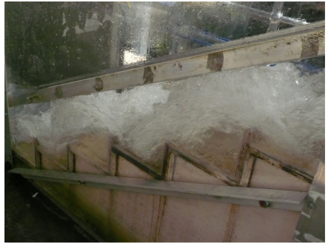
(B) d_c/h = 0.44 , Q = 0.015 m 3 /s, Re = 1.15 \times 10^5
