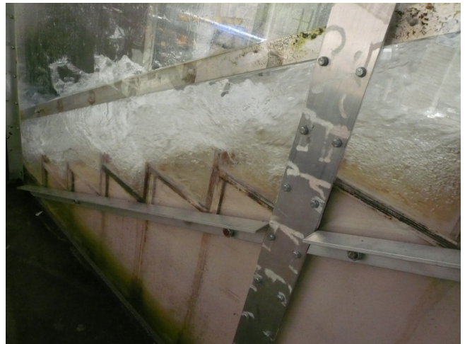
(F) d_c/h = 0.66 , Q = 0.028\text{ m}^3/\text{s} , Re = 2.1 \times 10^5
