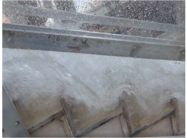
(B) d_c/h = 0.57 , Q = 0.022 m 3 /s, Re = 1.7 \times 10^5
