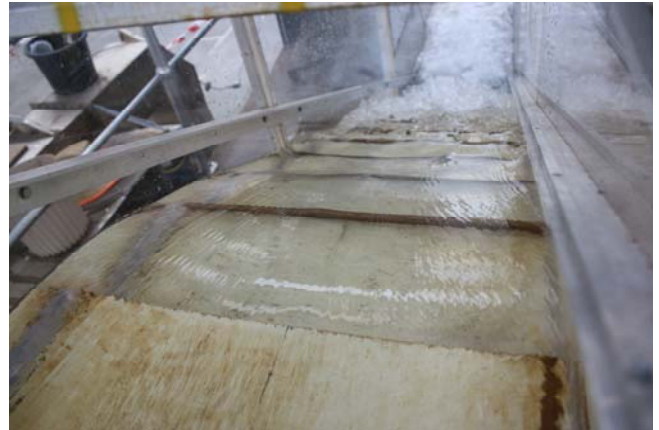
Fig. A-12 – Skimming flow regime on the pooled stepped spillway ( \theta = 26.6^\circ , w = 3.1 cm)
