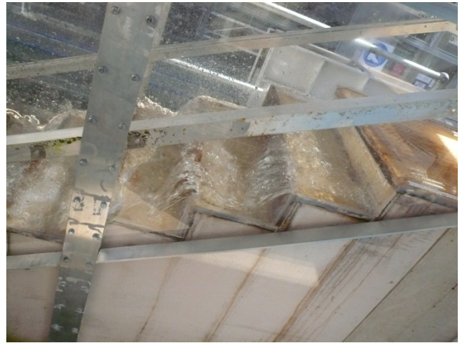
(B) d_c/h = 0.15 , Q = 0.003 m 3 /s, Re = 2.3 \times 10^4
