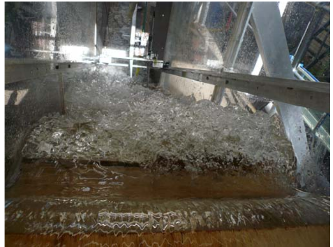
(B) dc/h = 0.50 , Q = 0.018 m 3 /s, Re = 1.4 \times 10^5
