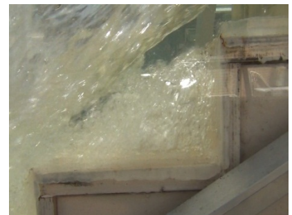
(B3) Distribution of air packet in cavity
