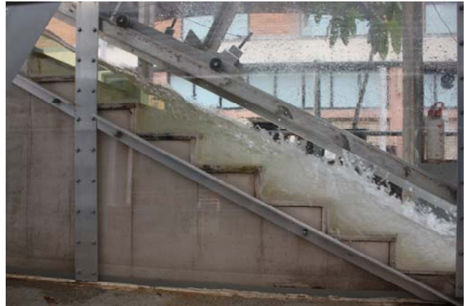
Fig. A-7 – Skimming flow regime on the flat stepped spillway ( \theta = 26.6^\circ )
