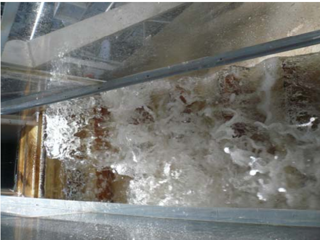
(E) d_c/h = 0.50 , Q = 0.018 \text{ m}^3/\text{s} , Re = 1.4 \times 10^5
