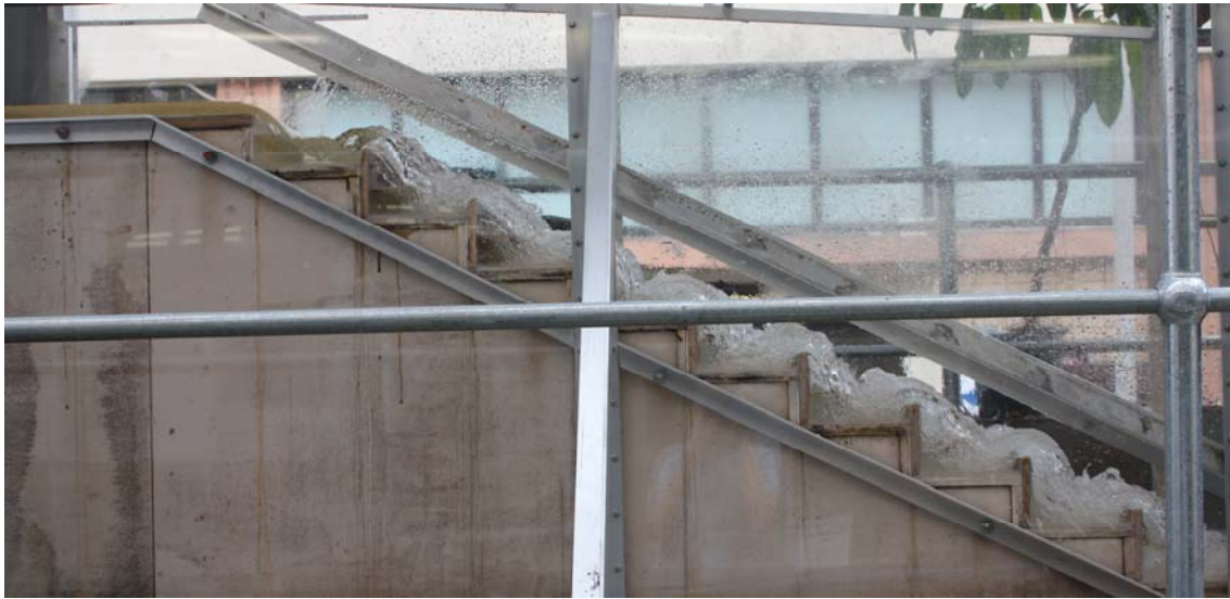
Fig. 3-2 –Nappe flow regime on pooled stepped spillway: d_c/h = 0.26 , Q = 0.007 \text{ m}^3/\text{s} , Re = 5.1 \times 10^4
