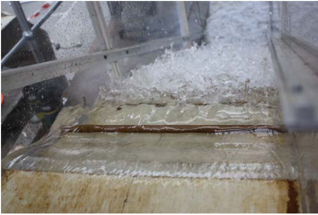
Fig. A-10 – Transition flow regime on the pooled stepped spillway ( \theta = 26.6^\circ , w = 3.1 cm)
