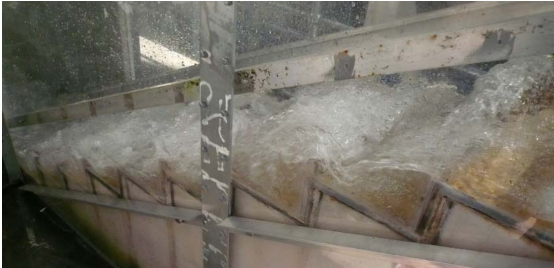
Fig. 3-11 - Nappe flow regime on the stepped spillway with staggered configuration of flat and pooled steps ( \theta = 26.6^\circ )
