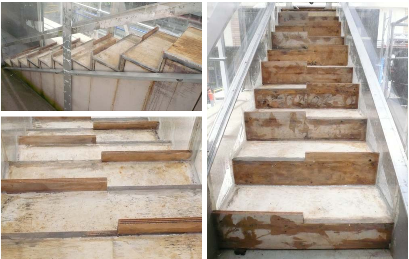
Fig. A-4 – Photos of the experimental setup of the stepped spillway with staggered configuration of flat and pooled steps ( \theta = 26.6^\circ )
