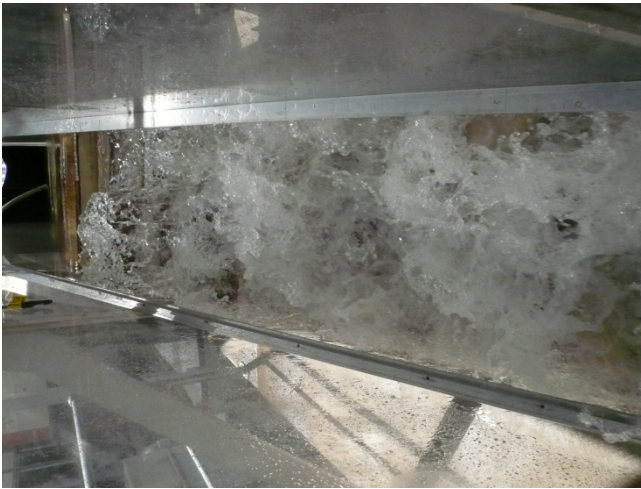
(A) d_c/h = 0.59 , Q = 0.023\text{m}^3/\text{s} , Re = 1.8 \times 10^5
