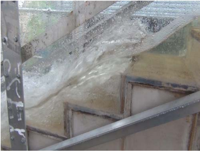
(C) d_c/h = 0.65 , Q = 0.027 m 3 /s, Re = 2.1 \times 10^4
