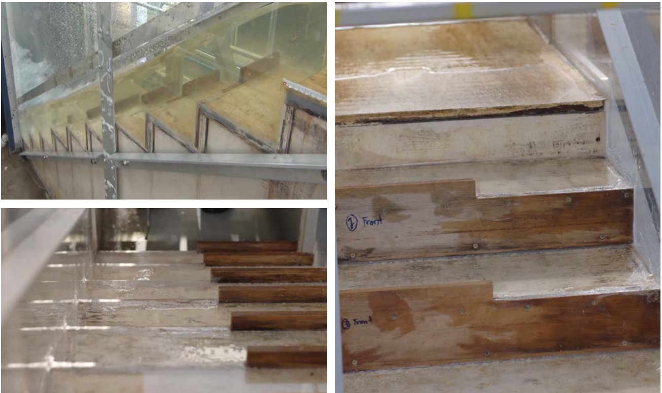
Fig. A-3 – Photos of the experimental setup of the stepped spillway with in-line configuration of flat and pooled steps ( \theta = 26.6^\circ )
