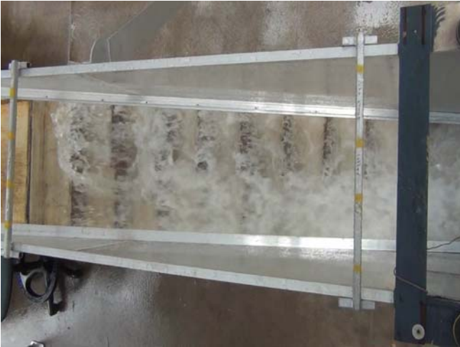
Fig. A-15 –Nappe flows (pooled step side) and transition flows (flat side) on the stepped spillway with in-line configuration of flat and pooled ( w = 3.1 cm) steps ( \theta = 26.6^\circ ) for 0.46 \leq d_c/h \leq 0.55 (A) d_c/h = 0.46 , Q = 0.016\text{m}^3/\text{s} , Re = 1.2 \times 10^5 (B) d_c/h = 0.46 , Q = 0.016\text{m}^3/\text{s} , Re = 1.2 \times 10^5
