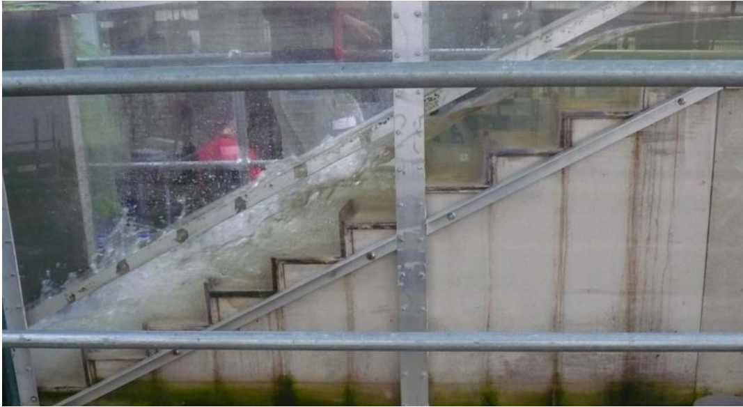
Fig. 3-13 – Skimming flow regime on the stepped spillway with staggered configuration of flat and pooled steps ( \theta = 26.6^\circ ): d_w/h = 1.45 , Q = 0.090 \text{ m}^3/\text{s} , Re = 6.9 \times 10^5
