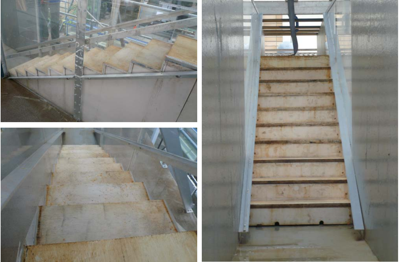
Fig. A-1 – Photos of the experimental setup of the flat stepped spillway ( \theta = 26.6^\circ )
