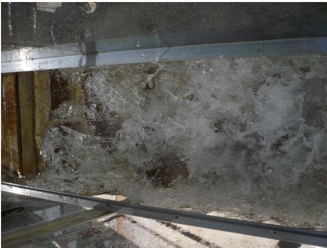
(E) d_c/h = 0.66 , Q = 0.028\text{ m}^3/\text{s} , Re = 2.1 \times 10^5
