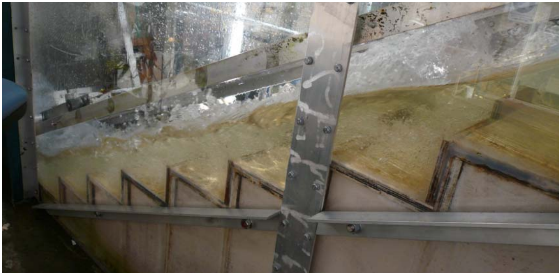
Fig. 3-9 – Skimming flow regime on the stepped spillway with in-line configuration of flat and pooled steps ( \theta = 26.6^\circ ): d_o/h = 1.15 , Q = 0.063 \text{ m}^3/\text{s} , Re = 4.9 \times 10^5
