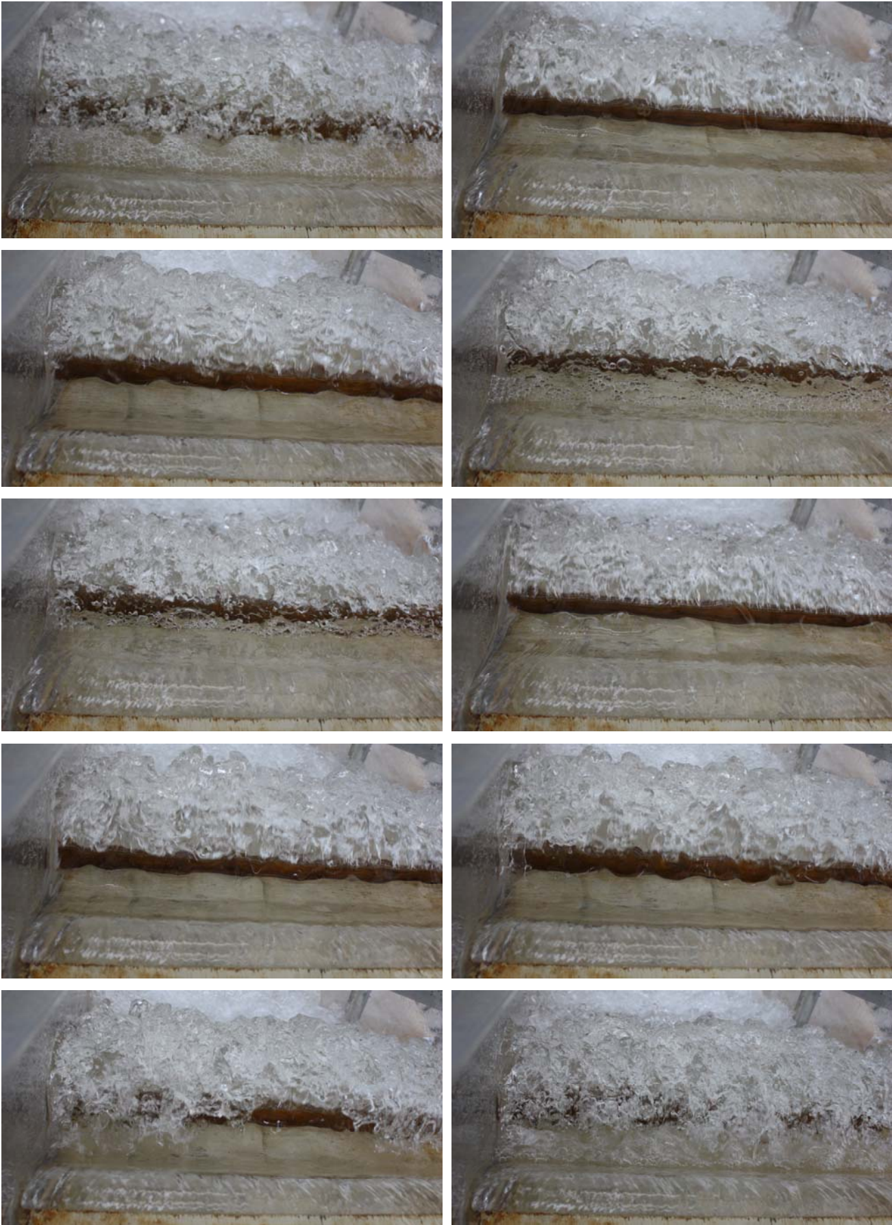
Fig. A-9 – Pulsations in first step cavity in the nappe flow regime on the pooled stepped spillway ( \theta = 26.6^\circ , w = 3.1 cm): d_c/h = 0.40 , Q = 0.013 m 3 /s, Re = 1 \times 10^5 (order from top left to bottom right)
