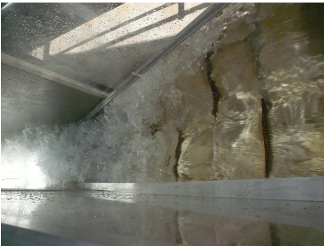
(E) d_c/h = 1.80 , Q = 0.124 \text{ m}^3/\text{s} , Re = 9.5 \times 10^5
