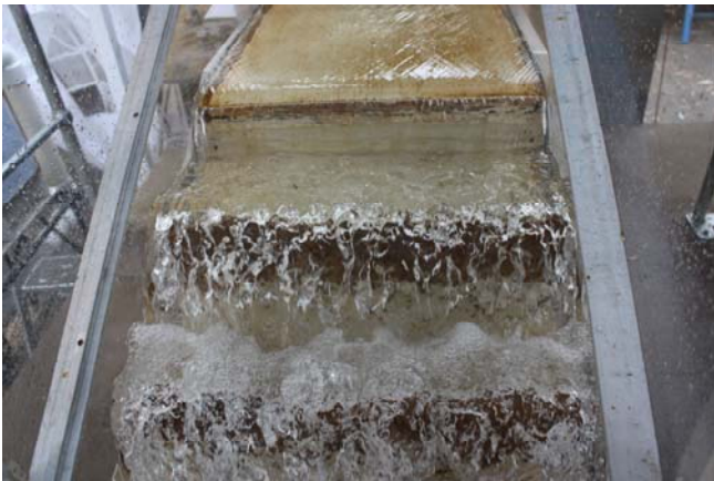
Fig. A-8 – Nappe flow regime on the pooled stepped spillway ( \theta = 26.6^\circ . w = 3.1 cm)
