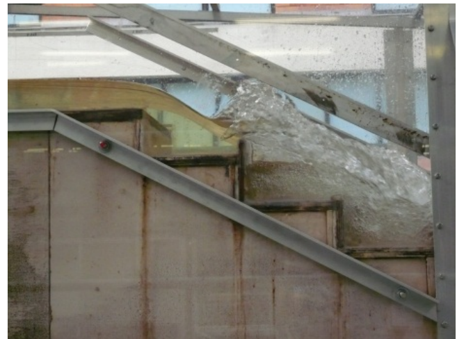
(D) Standing sidewall waves, d_c/h = 0.59 , Q = 0.023 \text{ m}^3/\text{s} , Re = 1.8 \times 10^5
