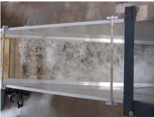
(C) dc/h = 0.55 , Q = 0.021 m 3 /s, Re = 1.6 \times 10^5
