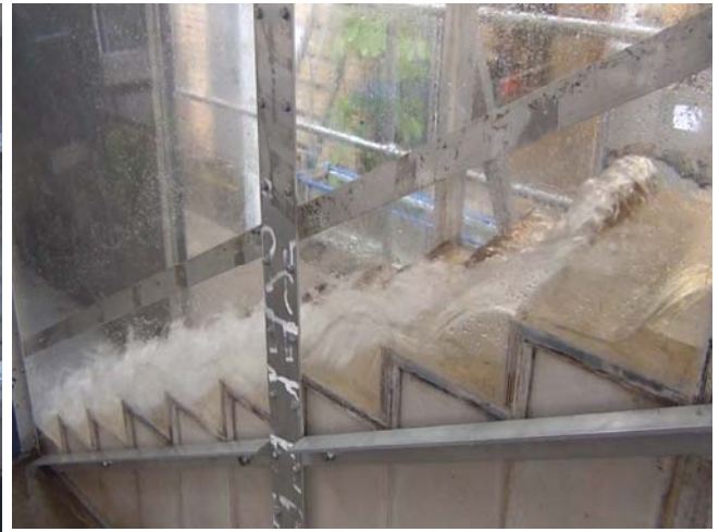
Fig. A-13 – Nappe flow regime on the stepped spillway with in-line configuration of flat and pooled (w = 3.1 cm) steps ( \theta = 26.6^\circ )
