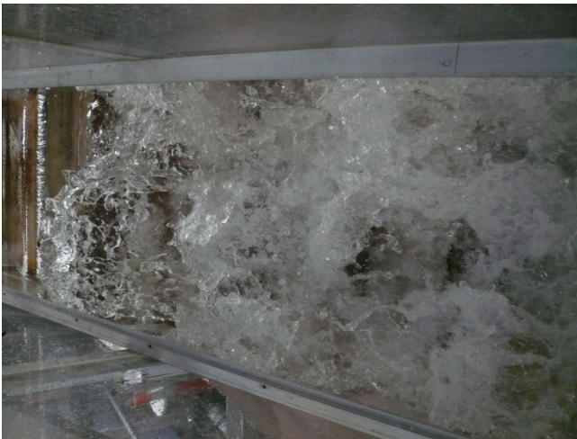
(C) d_c/h = 0.56 , Q = 0.020 m 3 /s, Re = 1.64 \times 10^5
