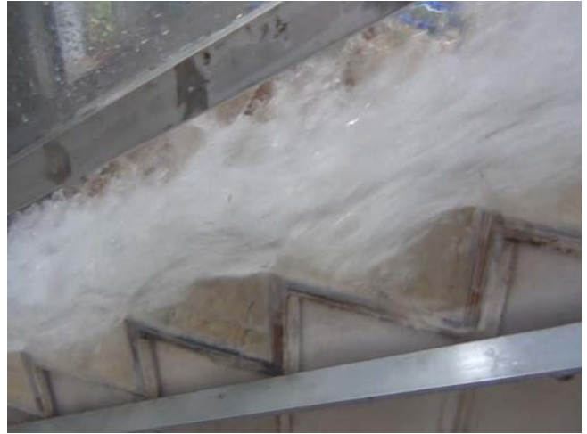
Fig. A-14 – Nappe flow regime on the stepped spillway with in-line configuration of flat and pooled (w = 3.1 cm) steps ( \theta = 26.6^\circ )
