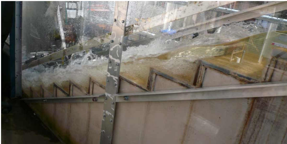
Fig. 3-8 – Transition flow regime on the stepped spillway with in-line configuration of flat and pooled steps ( \theta = 26.6^\circ ): d_o/h = 0.70 , Q = 0.030 \text{ m}^3/\text{s} , Re = 2.30 \times 10^5
