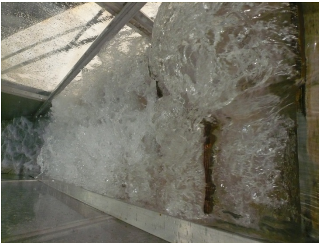
(C) d_c/h = 0.59 , Q = 0.023\text{m}^3/\text{s} , Re = 1.8 \times 10^5
