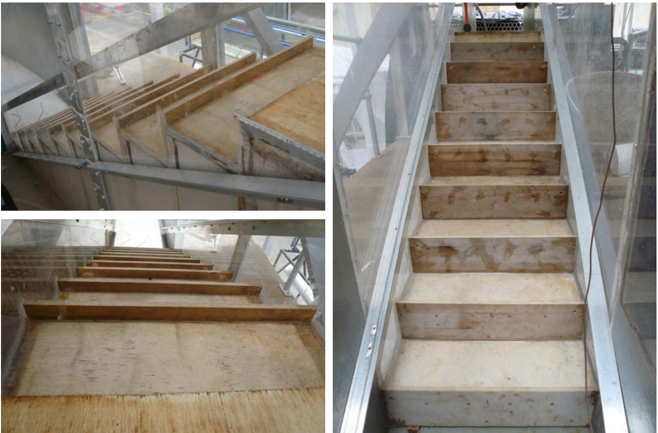
Fig. A-2 – Photos of the experimental setup of the pooled stepped spillway ( \theta = 26.6^\circ )
