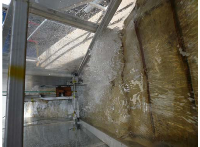
(B) d_c/h = 1.15 , Q = 0.063 m 3 /s, Re = 4.9 \times 10^5
