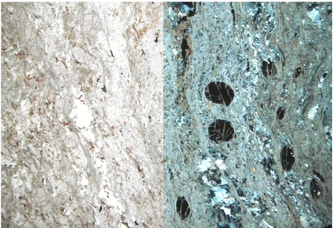
Photographs of thin sections for MLNB1 (Top) MLNS1 (Bottom). The right hand side of the image is with crossed polars.
