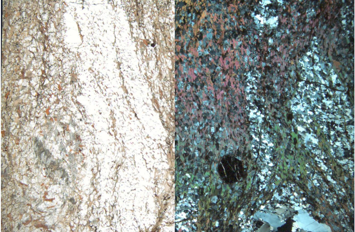
Photographs of thin sections for MLMR5 (Top) MLMR6 (Bottom). The right hand side of the image is with crossed polars.
