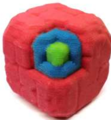
Figure 66. A 2.5 cm 3D-printed colored sandstone model of the core-sandwich-shell Pd-Ni-Pt nanocube.
