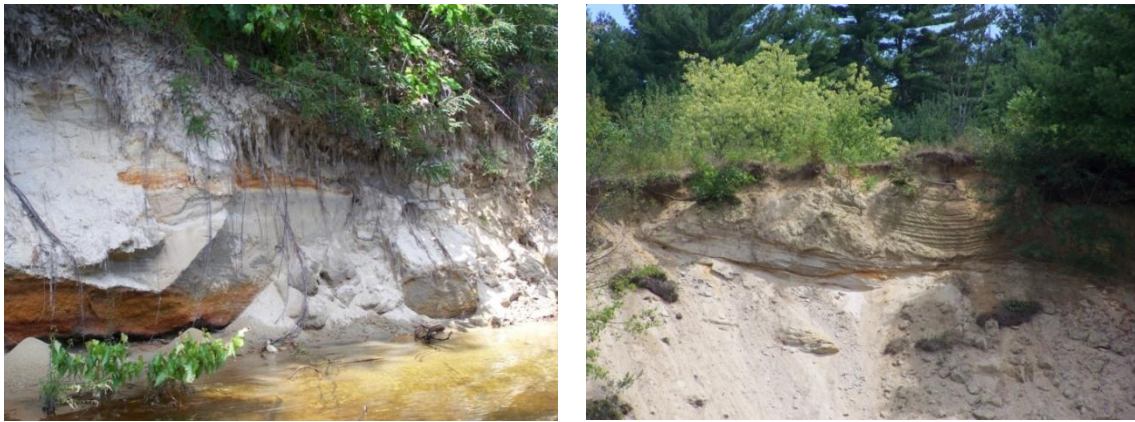
Figure 24: (Left) a ~0.5 m exposure of pebbly coarse sand located ~8.5 km upstream from Ayers Island Dam. (Right) deltaic sediment located at the Merrimack River boat ramp near Boscawen NH. Neither exposure had a clay-rich capping layer that would promote the buildup of pore-water pressure during earthquake shaking.
