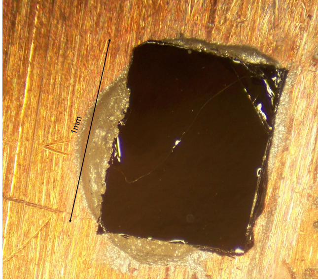
Figure 3.10: Photograph of a cleaved \text{Bi}_2\text{Sr}_{2-x}\text{La}_x\text{CuO}_{6+\delta} , glued with conducting epoxy to a copper sample holder. The samples we use are typically 1mm square.
