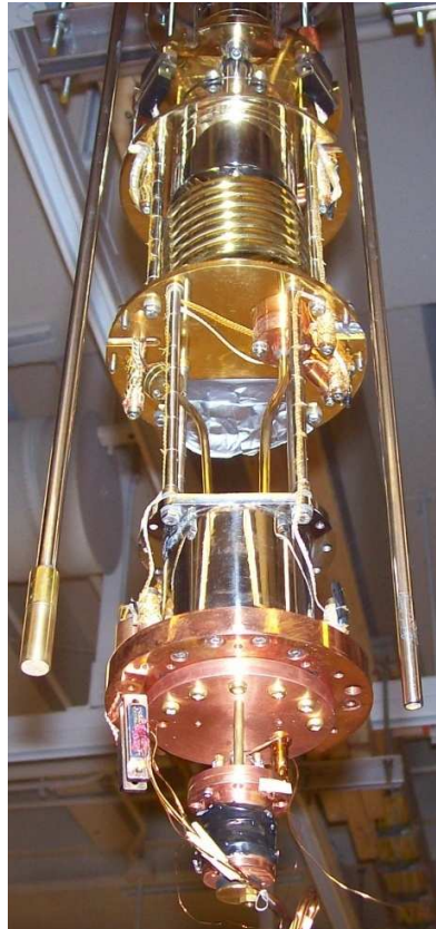
Figure 30: Photograph of the dilution refrigerator that would be used for this experiment. The calorimeter in which the sample is housed is depicted at the bottom of the image and is connected to the heat exchanger. The mixing chamber is the silver cylinder connected to the heat exchanger.
