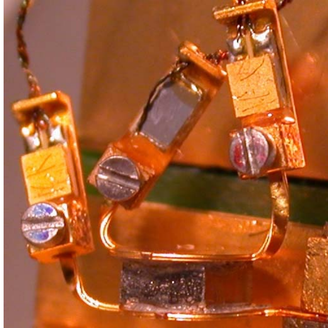
Figure 3.2: Image of a sample measured using the Thermal Transport Option of the PPMS.
