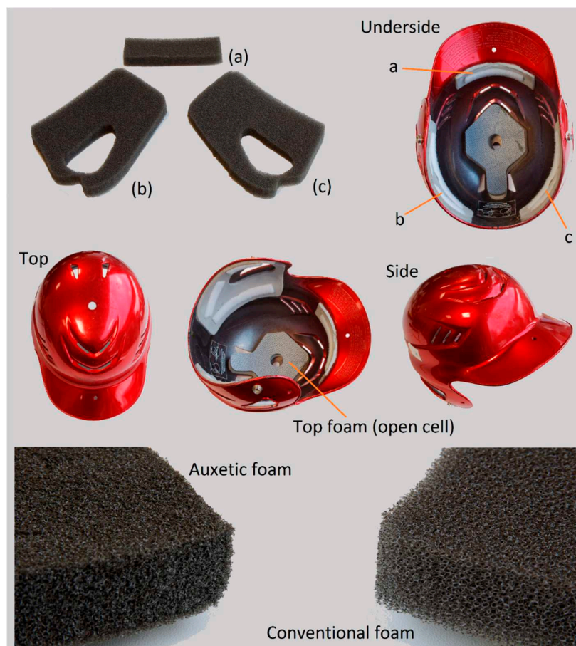
Figure 1. Foam inserts: (a) forehead, (b) right side, and (c) left side and views of the helmet showing native closed cell EVA foam and the top open cell foam in situ along with markers showing where inserts are placed. Also showing the foam structures for the auxetic (bottom left) and conventional (bottom right).
