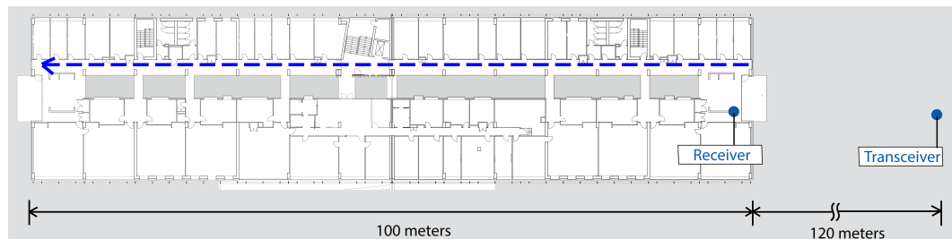
Figure 6.39: The placement of the transceiver, the control receiver (in the case of the measurement E1 or F1) or the second receiver (in case of the measurement E2 or F2) and the path of the moving transceiver. The transceiver positioned outside the building was placed 2 meters above the ground, while the receiver on the third floor of the building was placed near the window at the height of 2 meters.
