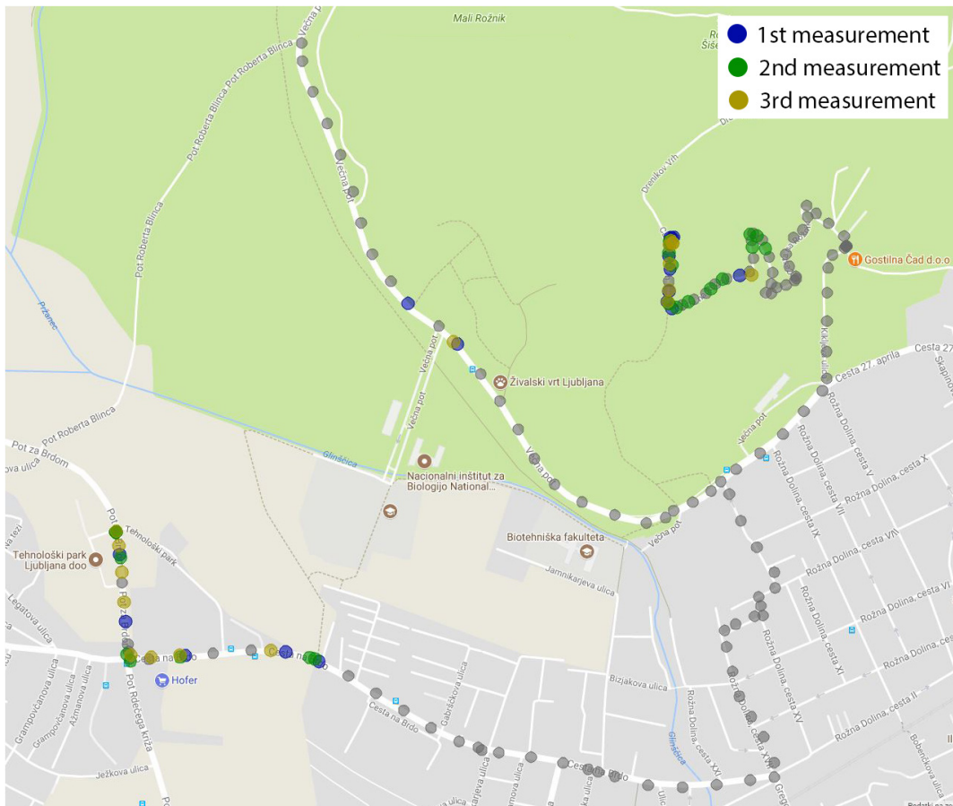
Figure 6.69: This map shows the area where the packets were received (the green, blue and yellow dots) and the places where there was no reception during the measurement G1.
