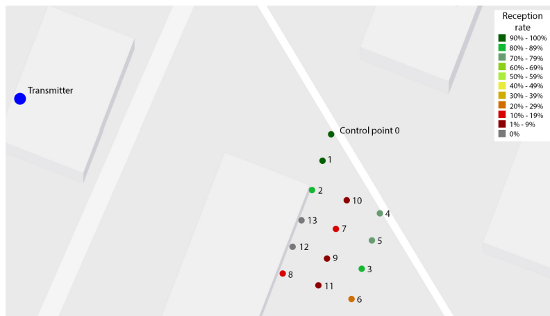
Figure 6.8: The measurement A: The placement and the reception rate of each node when the transmitter was positioned on the far side of the adjacent building. The point numbers are ordered (descending) by the reception rate.
