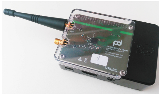
Figure 5.2: Our Raspberry Pi 3 Model B with a custom LoRa module and a 868 MHz antenna connected to a high-frequency connector.
