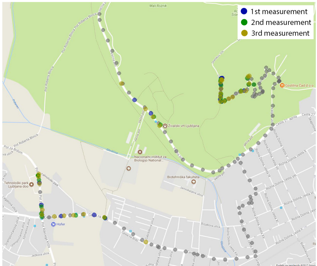
Figure 6.70: This map shows the area where the packets were received (the green, blue and yellow dots) and the places where there was no reception during the measurement G2.
