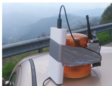
Figure 6.1: The receiver (the Raspberry PI 3 Model B) placed on the car roof (the rotary light was used just for the easier fixing of the receiver and power bank to the roof).
