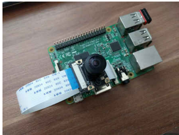
Figure 8 Raspberry Pi 2 model B computer with a camera module is used in the latest implementation of the installation ‘15 seconds of fame’ (see online version for colours)
