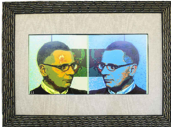
Figure 9 Monitors with about 2:1 aspect ratio enable the display of two square portraits side by side (see online version for colours)
