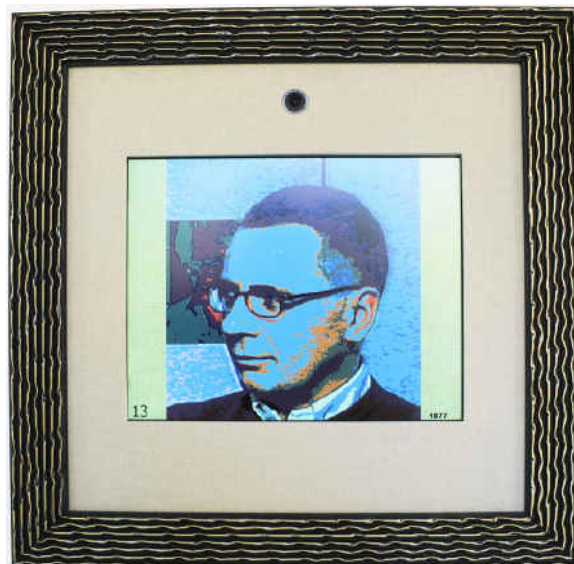
Figure 2 The original version of the installation ‘15 seconds of fame’ showing a flat computer display, framed as a painting with a round opening on top for the lens of the digital camera (see online version for colours)
