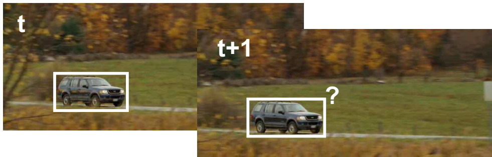
Figure 1.1: Main task in visual tracking: given two sequential frames from a video and the position of an object in t -th frame, the position of an object in frame t + 1 is estimated.
