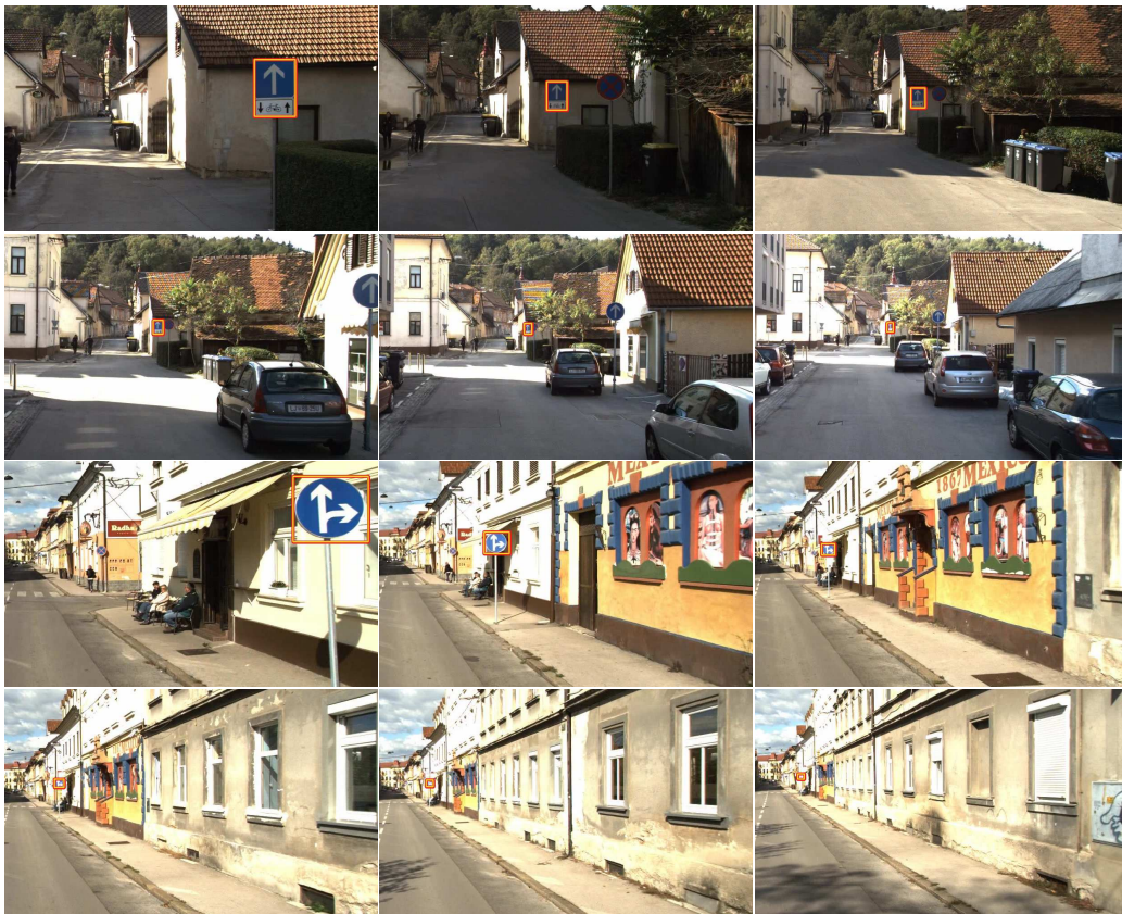
Figure 6.2: Visual tracking of the traffic signs with the camera mounted on a car in a mobile mapping system. The tracker is able to address the size change of the object even though it significantly changes during the tracking.
