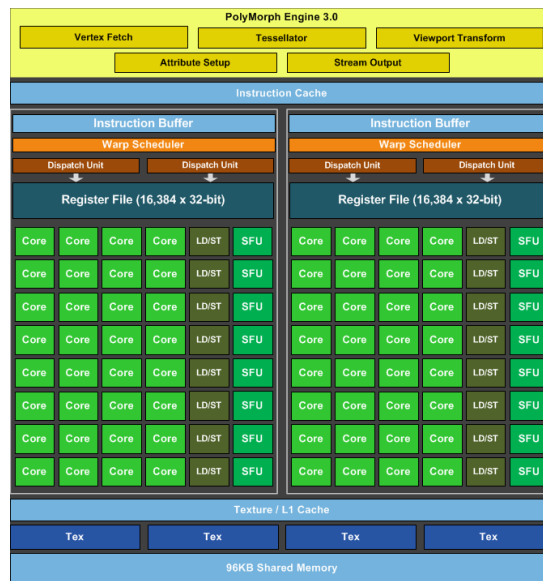
Figure 2.2: Streaming Multiprocessor Maxwell (figure source: [21]). All of the cores are meant for processing data. The figure has been cropped slightly and modified to show only two out of four warps.
