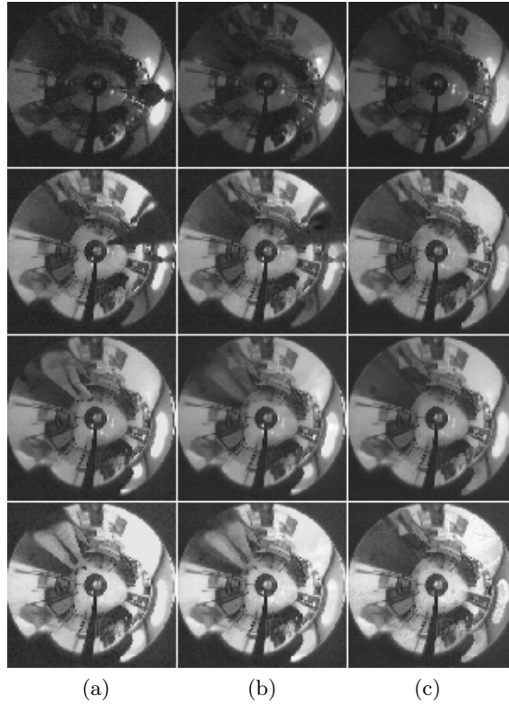
Fig. 4. (a) Four panoramic images from the sequence, (b) their reconstructions based on the standard PCA, and (c) their reconstructions based on the robust PCA.
