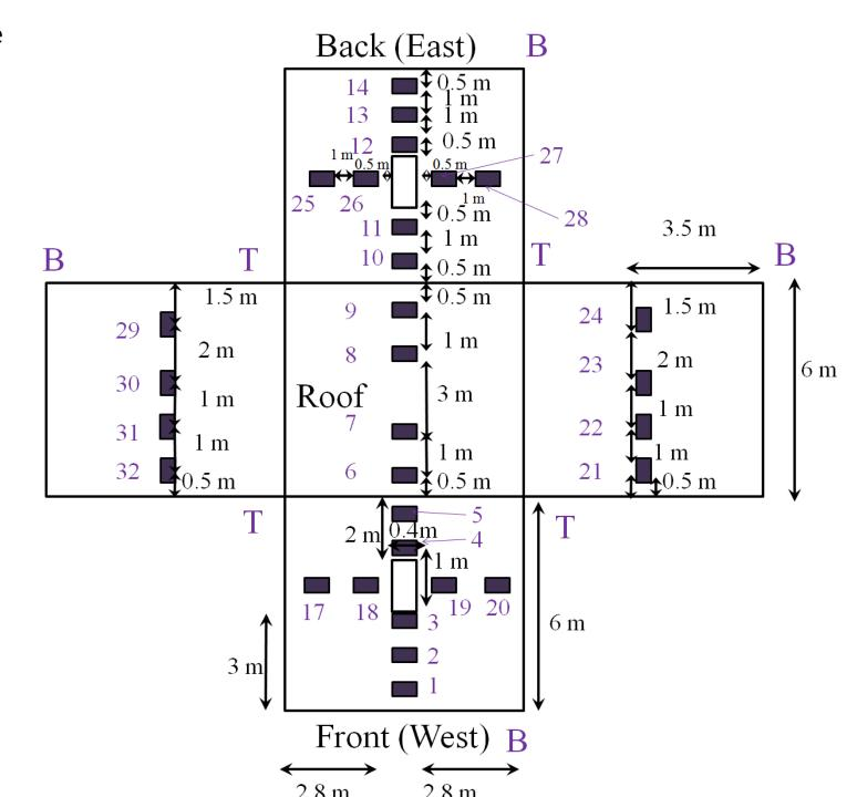
RCC full-scale study site at Silsoe: a) plan view with the main features (unchanged since 2009), b) oblique view into the prevailing wind direction of the cube array, with sonic anemometer locations, storage shed (black diamond) and sewage tanks (black triangle), c) plan of the site with angle notation. The blue cube in (b) and square in (d) is the instrumented cube. All cubes are 6 m by 6 m x 6 m. Sources of a: Copyright 2016 Infoterra, Blue Sky Limited and Google Earth.
