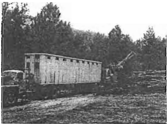
Figure 27.—“Utilizer” being tested in the Southwest which converts much of the logging residues normally left in the woods into chips for transport to the pulpmill.
