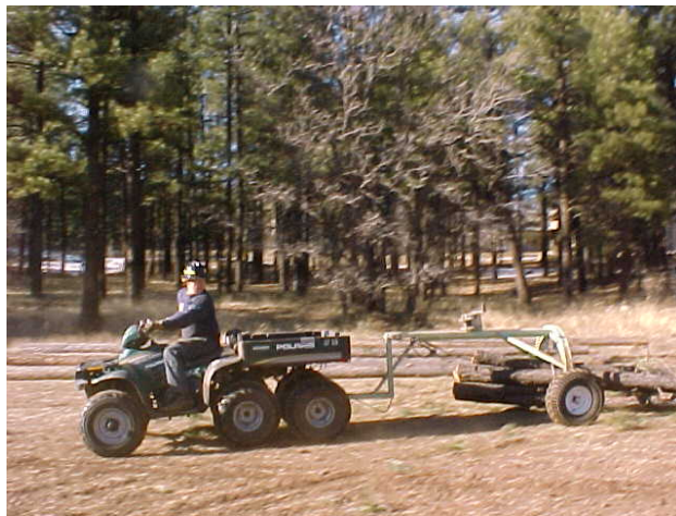
Photo 7 – “Micro” harvesting: Skidding wood with an ATV (Roll-over protection recommended for this type operation)
