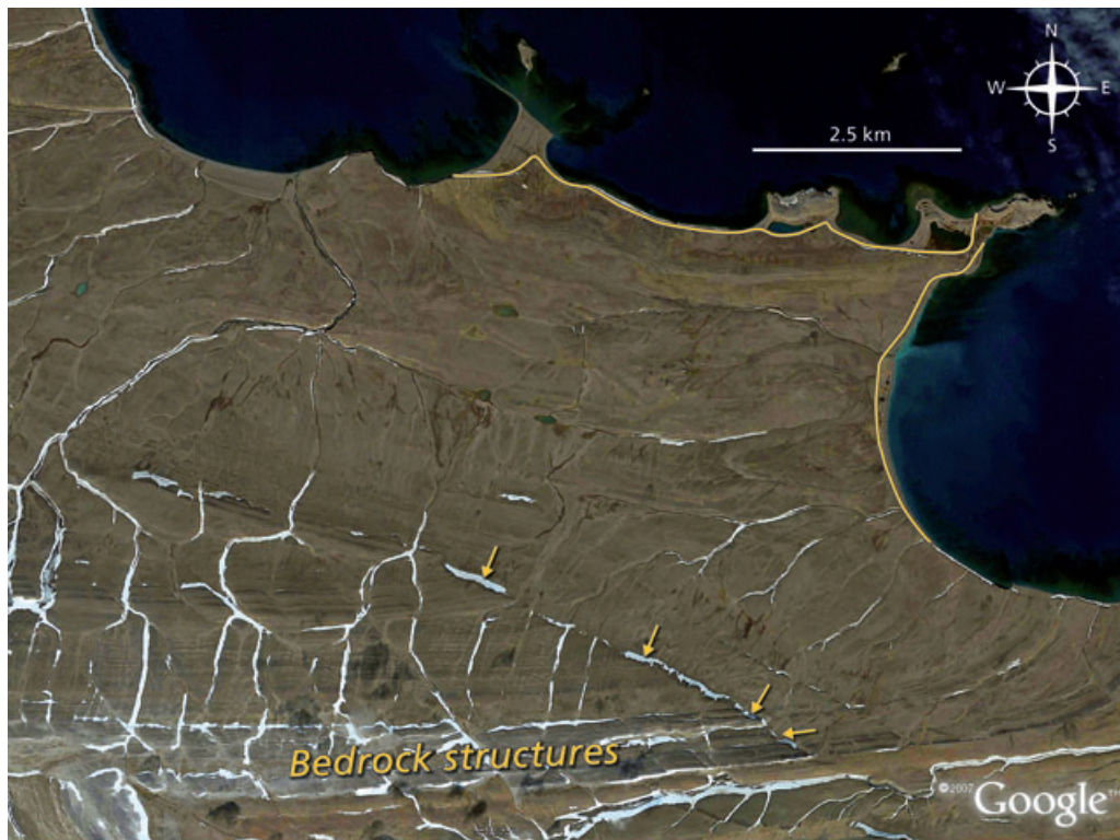
Fig. 7 Satellite image downloaded from Google Earth Professional on 15 November 2007 (image credit: Google Earth™ mapping service). Arrows show a shoreline at about 140 m a.s.l. cutting bedrock structures. Above the shoreline the bedrock is completely exposed; below there is a thin cover of unconsolidated sediments. We interpret the latter as beach and shallow marine sediments subsequently modified by an ice sheet, and then by solifluction. Lower shorelines can be discerned in places. The thin yellow line shows the postglacial marine limit, about 10 m a.s.l., from Zeeberg et al. (2001).
