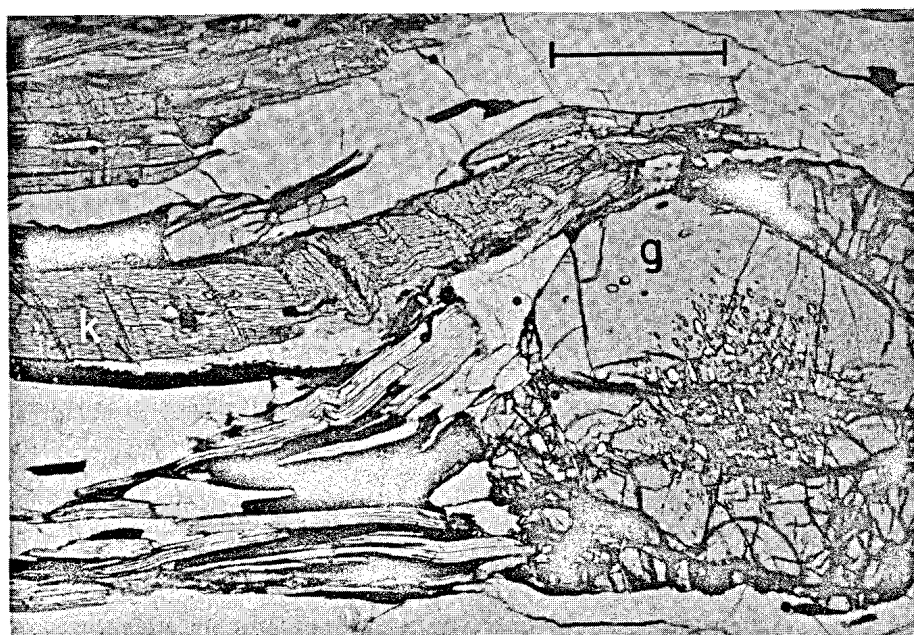
Fig. 2. Kink folds in kyanite (k) buttressed by a garnet (g) crystal, from sample CC-32a (Monarch Canyon, location in Figure 1). Plane-polarized light. Scale bar is 1 mm long.
