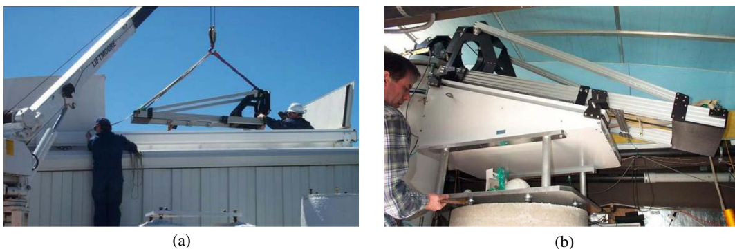
Fig. 4 Simple mechanical test fit of beam compressor mount in astrometric station. (a) Compressor being lowered into astrometric station. (b) Compressor fitted to concrete pier between fast tip-tilt mirror (upper left) and siderostat (outside view to right) at the 20-deg down-tilt operational angle.
