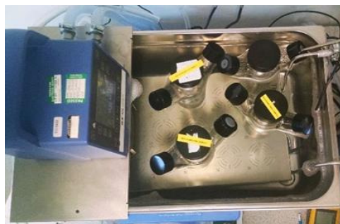
Figure 1. Experimental setup for sonocrystallization experiments in the XUB25 ultrasonic bath
