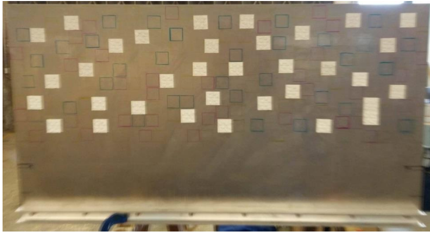
Fig. 4 – 10% coverage area of barnacles on flat plate
