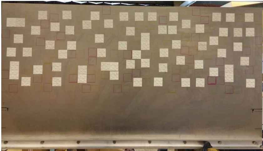
Fig. 5 – 20% area coverage of barnacles on flat plate
