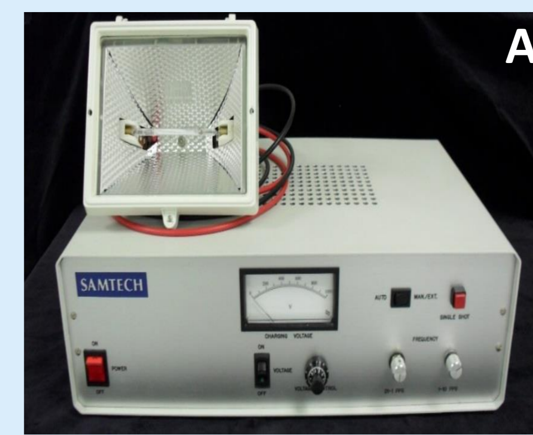
Fig 2. Xenon filled flash lamp and pulsed power generator and (B) UV-rich emission spectrum of xenon flash lamp.
