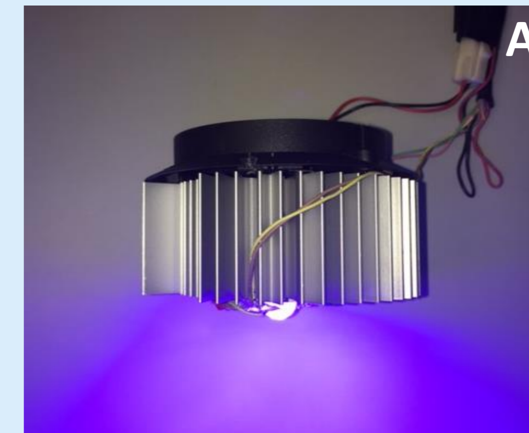
Fig 1. 405 nm LED array and (B) optical emission spectrum of 405 nm LED array.
