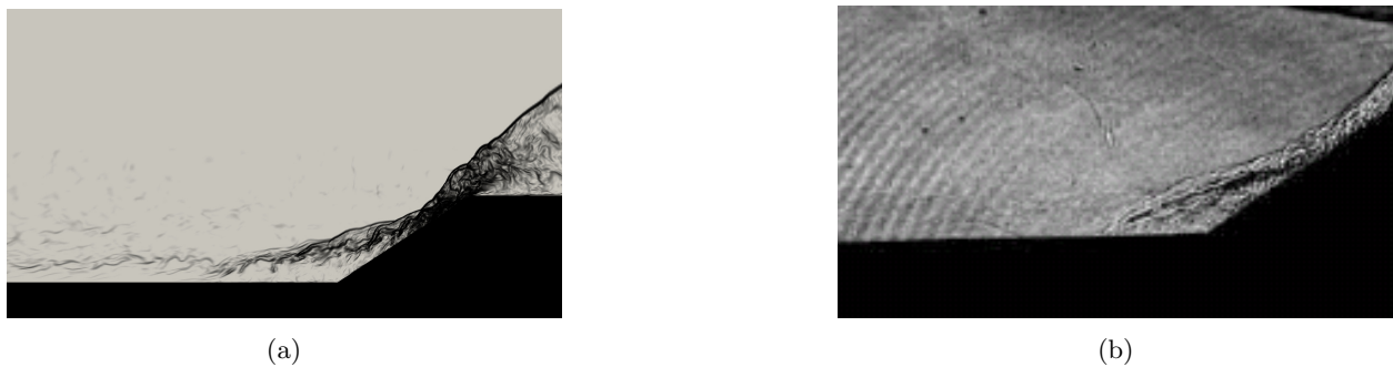
Figure 8: Qualitative comparison between iLES and experimental data. (a) Instantaneous numerical Schlieren ( NS = 0.8 * \exp(-0.1|\nabla\rho|) ) of the ramp area. (b) Schlieren image of the Mach 7.2 SWBLI experiment by Wadhams et al. 22
